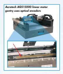
One of the major benefits of using a linear encoder system in a linear motor setup is that the reading head and scale can be placed very close to or at the bearing centerline, where it will measure the linear position at its most accurate point - i.e., free from Abbe errors that are caused by very small angular deviations in straightness and flatness being amplified by the distance between the bearing and the point of measurement.
