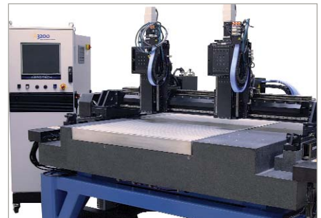
SolarScribe-GM with optional dual-carriage step axis, control cabinet, and isolation system.
