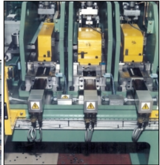
A view of several rollform axes and their servomotors
