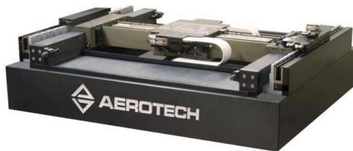
Figure 4. PlanarHD planar air bearing with exceptional geometric performance and \pm 50 nm long-term repeatability.
