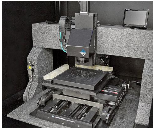
Figure 3. An XY positioning system using interferometer feedback at the working plane to minimize abbe error influences at the work point.
