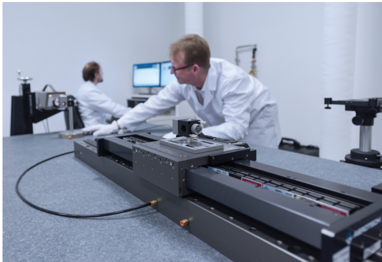
Figure 1. Metrology technician setting up laser interferometer testing.
