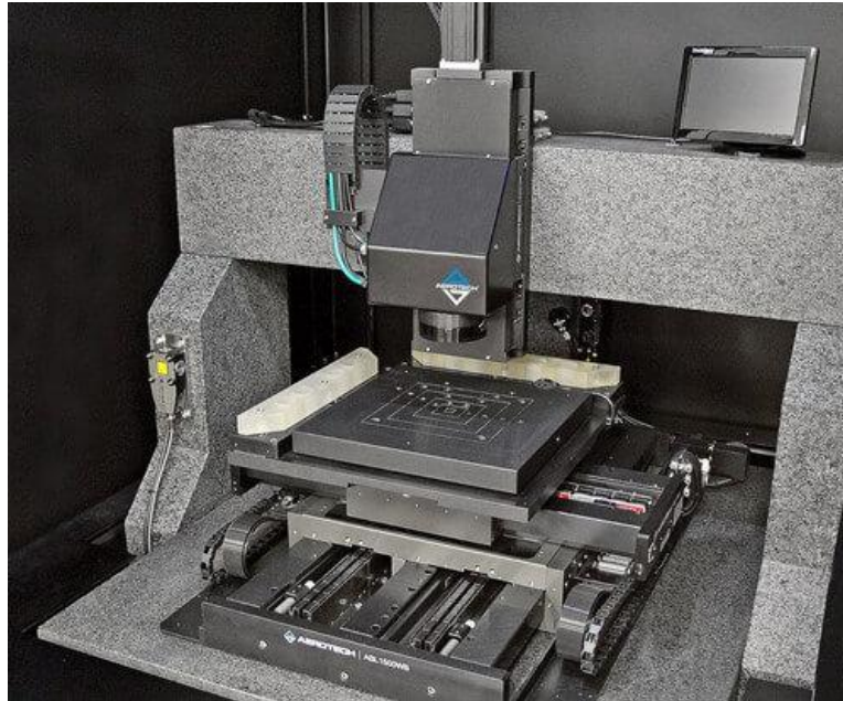
Figure 21. A 2D laser interferometer system that is being used to compensate for Abbe error offsets and on-axis accuracy in real time.
