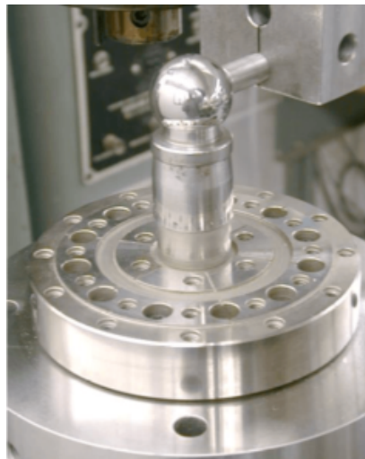
Figure 16. A precision test artifact (the ball) and the capacitive probe.
