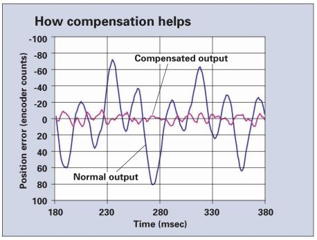
Software-based compensation offers almost an order of magnitude improvement in cogging compared to uncompensated motor output.
