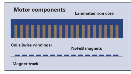
Slotted linear motors consist of a magnet track and a wire wound iron core. The iron helps channel and focus magnetic flux, increasing flux density, which results in higher force.
