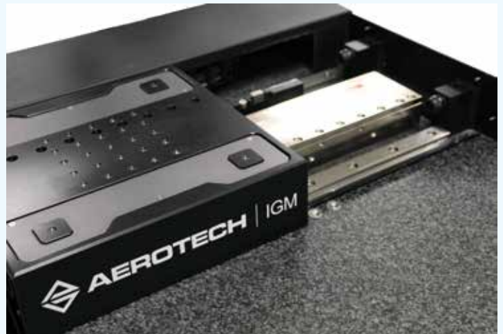
Motion components, such as bearing rails, motors, and feedback devices, are mounted directly to the main granite structure.
