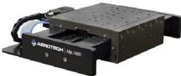
Air bearings are normally used for very high-precision applications where the friction-free characteristics of the bearing perfectly complement the noncontact linear motor and feedback device design, allowing the very best positioning performance. Air bearings typically rely upon a very small air gap of just a few microns with
