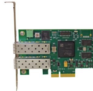
SFP ports for the glass optical fiber, high-speed HyperWire communication bus and can connect up to 32 axes of precision motor drives — each capable of operating at industry-leading performance levels.
