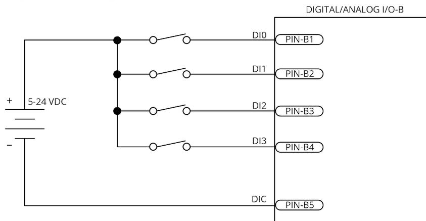
**Figure 2-10: Digital Inputs Connected to Current Sinking Devices**
