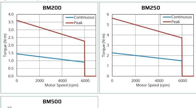
Figure 1-2: Torque Speed Curves (BM200, BM250, and BM500)
