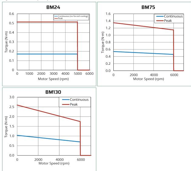
Figure 1-1: Torque Speed Curves (BM24, BM75, and BM130)
