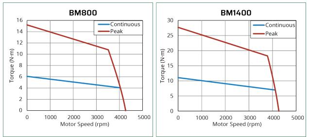
Figure 1-3: Torque Speed Curves (BM800 and BM1400)
