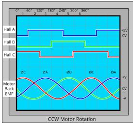
During CCW motor rotation, each Hall effect signal is at a logic low state when its corresponding motor phase is at a negative voltage.
