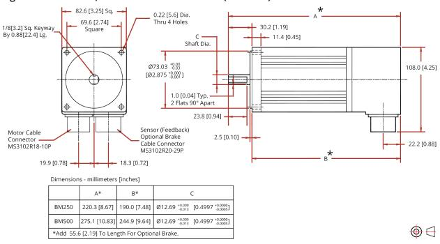
Figure 1-8: BM250, BM500 Model Dimensions (NEMA 34)
