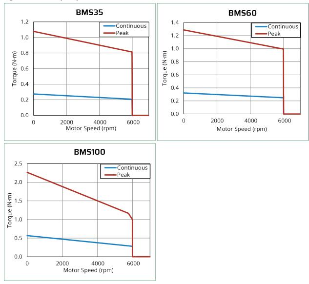
Figure 1-4: Torque Speed Curves (BMS35, BMS60, and BMS100)
