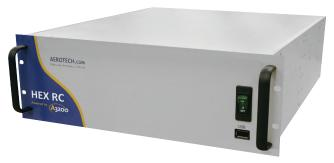
The HEX RC is ideal for controlling six-axis robotic systems like the Aerotech HexGen series hexapods.
