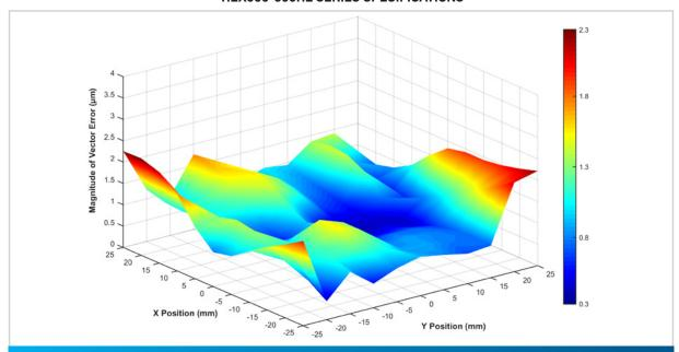
HEX500-350HL three-dimensional vector accuracy error measured when commanded to move in the XY plane at a Z position of 0 mm. The measurement was taken with three interferometers (X, Y, and Z directions) targeting a three-sided optic. The results show the outstanding three-dimensional accuracy capability of the HEX500-350HL.
