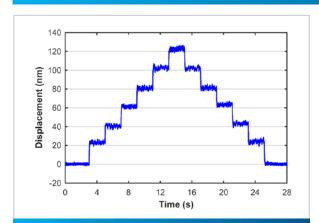
Minimum incremental step plot of the X-axis of the HEX500-350HL. All axes of the HEX500-350HL have industry-leading resolutions enabling higher-resolution processes.
