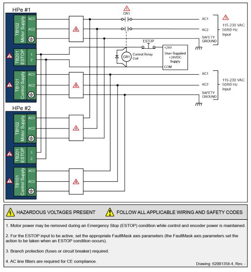
Figure 2-31: Typical Emergency Stop Circuit
