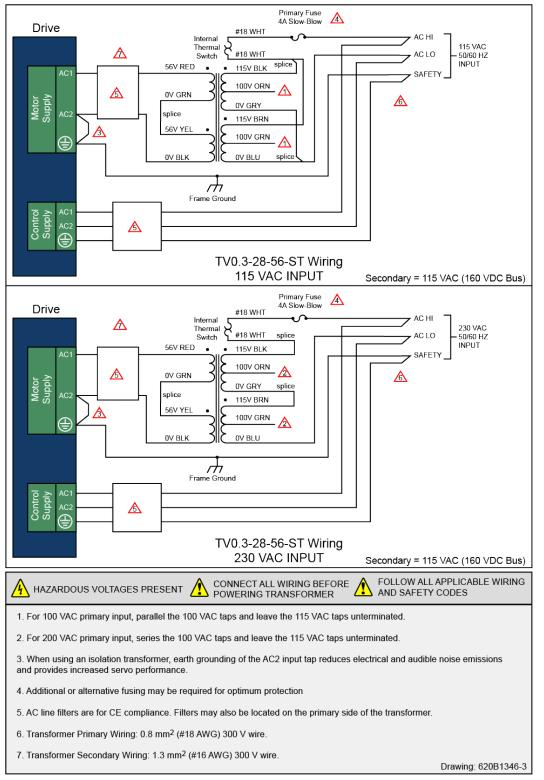
Figure 2-8: 160 Volt DC Bus from 115 and 230 VAC Source (TV0.3-56)
