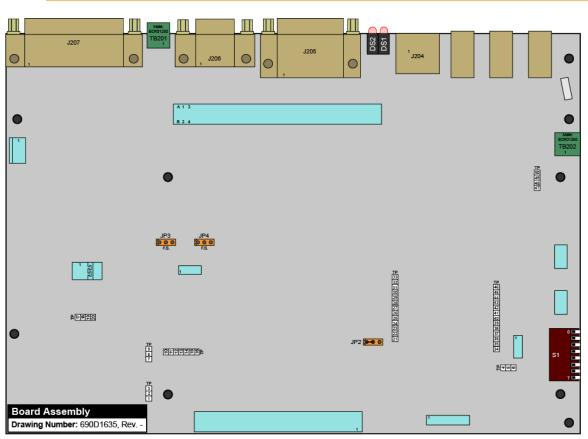
Figure 6-2: Control Board Assembly
