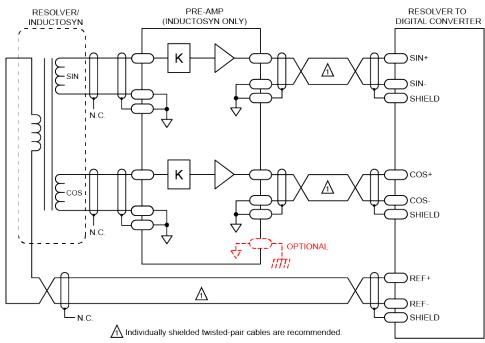
Figure 4-2: Resolver/Inductosyn Recommended Wiring
