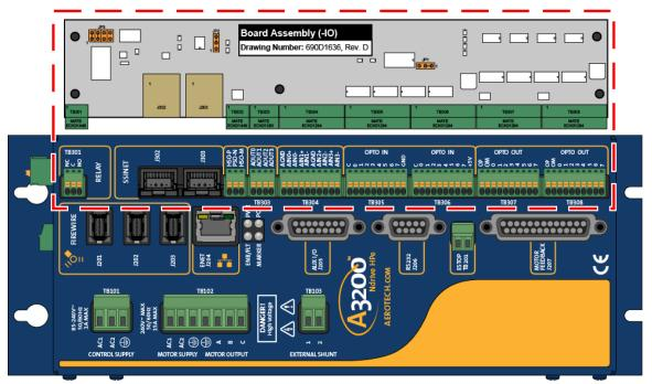
Figure 3-1: Ndrive HPe 10/20/30 with -IO Option Board
