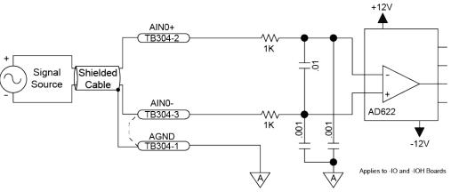
Figure 3-8: Analog Input Typical Connection (TB304)
