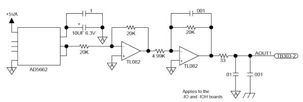
Figure 3-7: Analog Output Connector (TB303)
