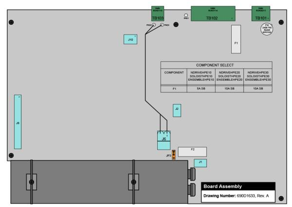
Figure 6-1: Power Board Assembly
