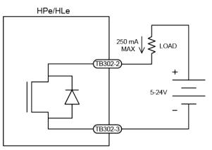
Figure 3-5: PSO Output Sinks Current
