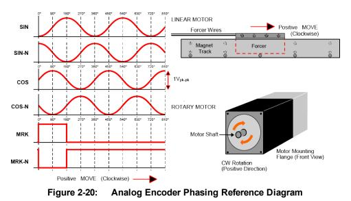
**NOTE:** The input amplitude is measured peak to peak for any encoder signal (sin, sin-n, cos, cos-n) relative to signal common. These signals have a typical offset voltage of 2V to 2.5V.
