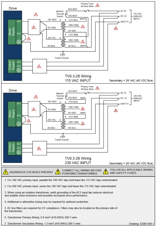
Figure 2-6: 40 Volt DC Bus from 115 and 230 VAC Source
