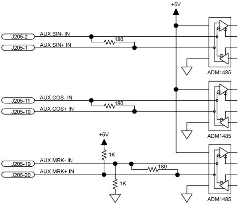
Figure 2-32: Auxiliary Encoder Channel (J205)
