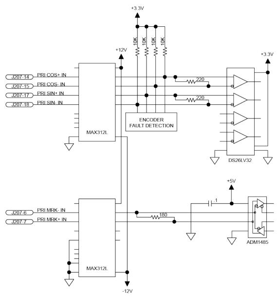
Figure 2-18: Line Driver Encoder Interface (J207)
