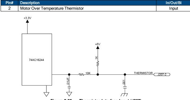
Figure 2-25: Thermistor Interface Input (J207)
