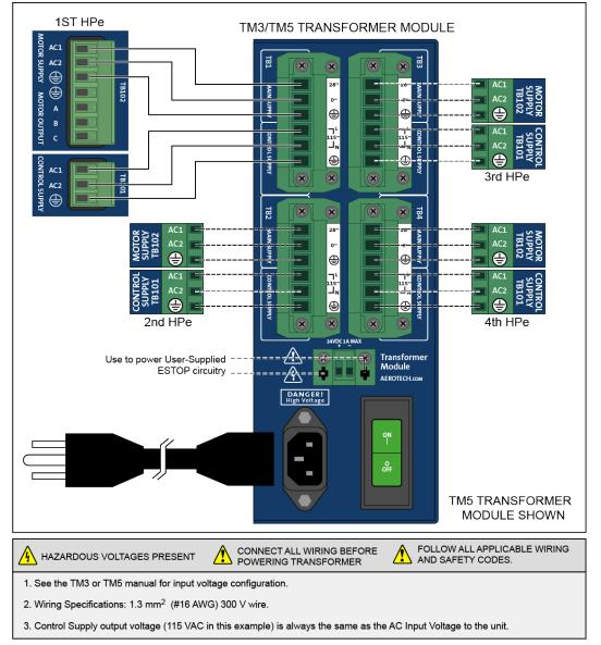
Figure 2-9: Control and Motor Power Wiring using a TM3 or TM5 Transformer
