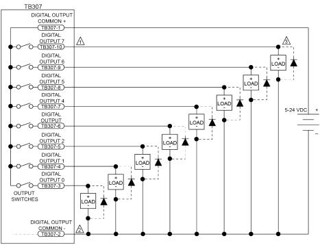
A DIODE REQUIRED ON EACH OUTPUT THAT DRIVES AN INDUCTIVE DEVICE (COIL), SUCH AS A RELAY.
