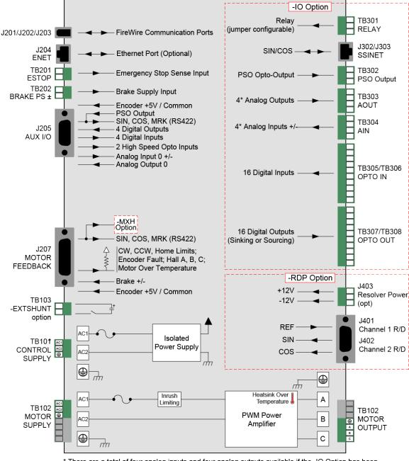
\* There are a total of four analog inputs and four analog outputs available if the -IO Option has been purchased.The analog I/O normally available on J205 is accessed through TB303 and TB304.
