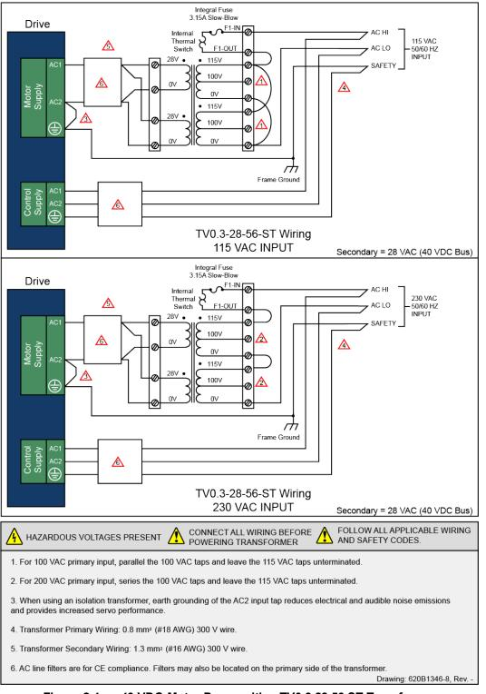
Figure 2-4: 40 VDC Motor Power with a TV0.3-28-56-ST Transformer
