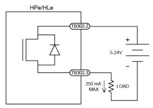
Figure 3-4: PSO Output Sources Current
