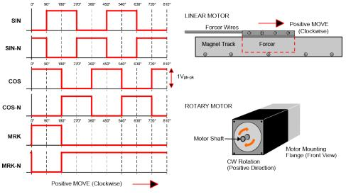
Figure 2-22: Encoder Phasing Reference Diagram (Standard)
