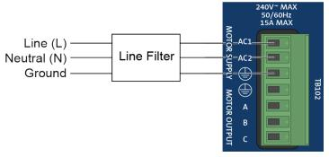
Figure 2-2: Motor Bus Input Connections
