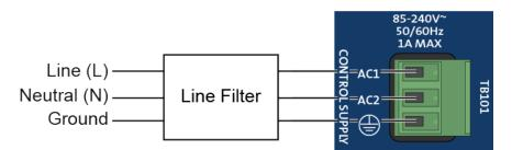
Figure 2-1: Control Supply Connections
