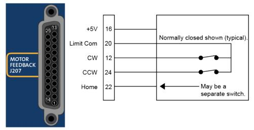
Figure 2-27: End of Travel Limit Input Connections
