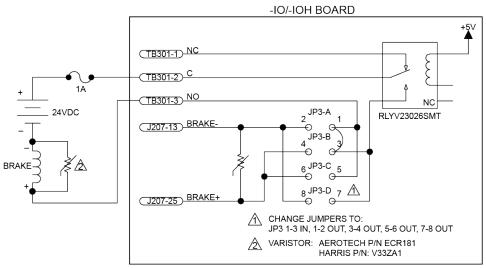
Figure 3-3: Brake Connected to TB301
