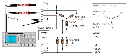
Figure 2-12: Motor Phasing Oscilloscope Example
