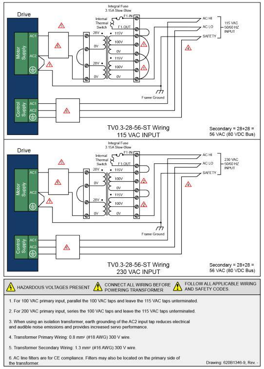
Figure 2-5: 80 VDC Motor Power with a TV0.3-28-56-ST Transformer
