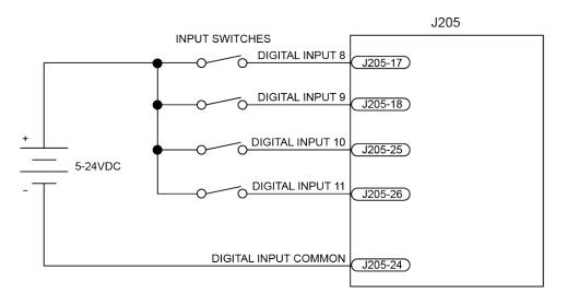
**NOTE:** Each bank of 8 Inputs must be connected in the all sourcing or all sinking configuration.
