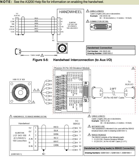
Figure 5-6: Handwheel Interconnection (to Aux I/O via a BBA32 Module)
