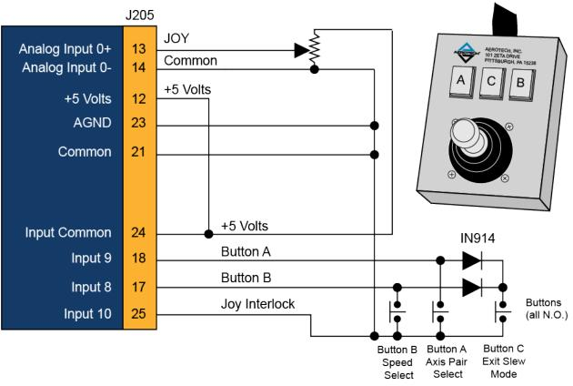
Figure 5-1: Single Axis Joystick Interface (to Aux I/O)
