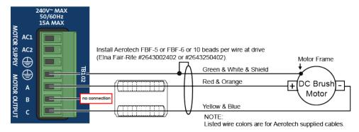
Figure 2-14: DC Brush Motor Configuration
