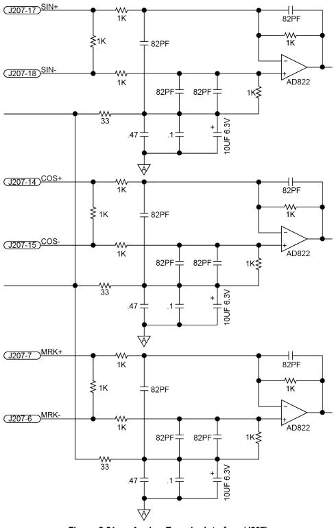
Figure 2-21: Analog Encoder Interface (J207)
