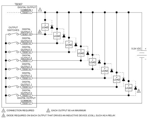
Figure 3-14: Digital Outputs Connected in Current Sinking Mode
