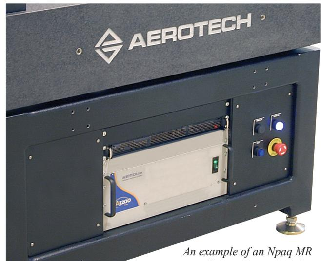
*An example of an Npaq MR installed in the machine base of a gantry system.*
