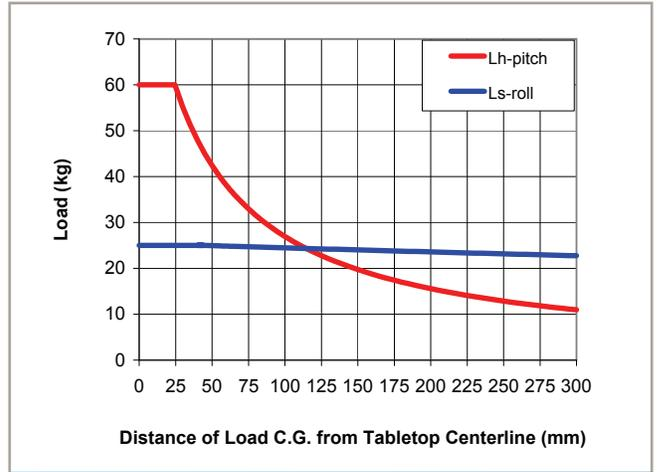
Cantilevered load capability (static conditions) for the ABL1500WB.
