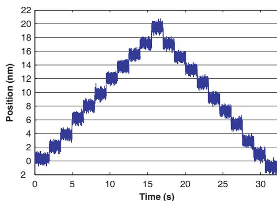
ANT130LZ-060-PLUS 2 nm step plot with 100 Hz filter.
