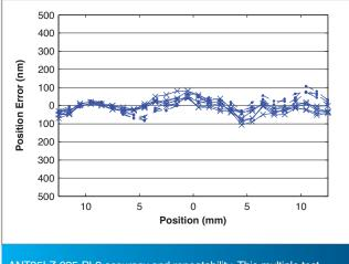
ANT95LZ-025-PL2 accuracy and repeatability. This multiple test run over an extended period of time shows the high level of system accuracy and repeatability.
