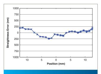
ANT95LZ-025-PL2 straightness error, five runs, bi-directional. Exceptional and highly repeatable – five times more accurate than the stated specification.
