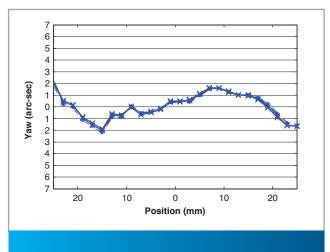
ANT95LZ-050-PL2 yaw, five runs, bi-directional. Highly repeatable, minimal yaw error enhances system positioning accuracy.
