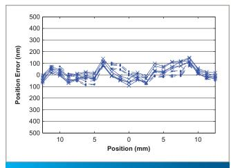
ANT95XY-025-PL3 accuracy and repeatability, five runs, bidirectional for the X (lower) axis. The total accuracy of 240 nm over 25 mm travel is significantly better than other offerings and half of its stated specification.
