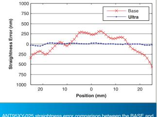
ANT95XY-025 straightness error comparison between the BASE and ULTRA models shows a dramatic improvement in this specification.
