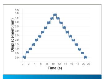
ANT95XY-025-E4 lower axis 0.5 nm step plot. Best-in-class resolution and exceptional in-position stability for large-travel stages.
