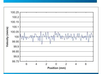
ANT95XY-025-PL3 velocity performance at 100 mm/s and 1 kg payload for the X (lower) axis. This outstanding speed stability enhances most scanning or laser machining applications.
