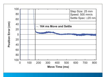
ANT95XY-025-PL3 step and settle performance at full travel and 1 kg payload for the X (lower) axis. Industry-best settling times significantly improve throughput for most applications.
