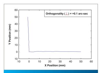
ANT95XY-050-PL4 orthogonality. The plot is exaggerated 10,000X for clarity. The ULTRA model orthogonality is a twenty-fold improvement over the BASE model orthogonality.
