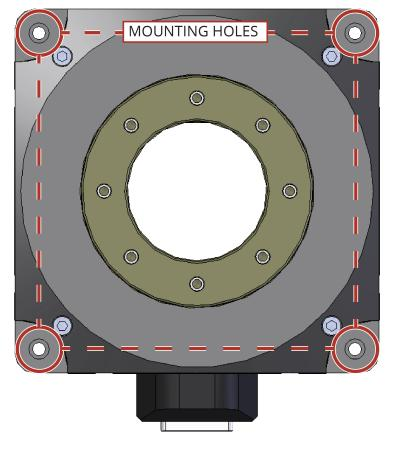
Figure 2-2: APR200DR Stage Mounting Holes
