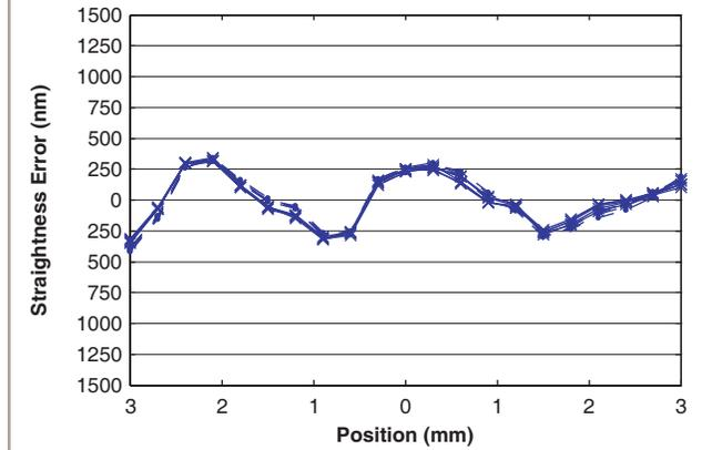
*ANT130V-5-PLUS straightness error; five runs, bi-directional, perpendicular to the wedge.*
