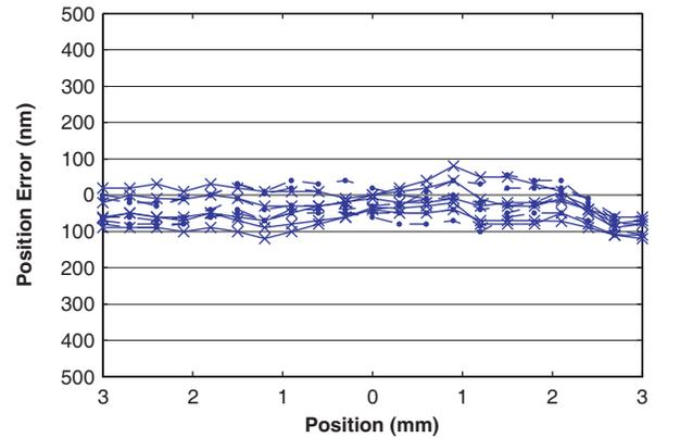
*ANT130V-5-PLUS accuracy and repeatability. This multiple test run over an extended period of time shows the high level of system accuracy and repeatability.*
