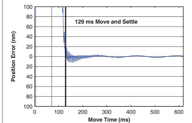
*ANT130V-5-PLUS step and settle performance at 75 mm/s, with a settle spec of  $\pm 20$  nm, and a step size of 5 mm. Outstanding settling time enhances throughput of most applications.*
