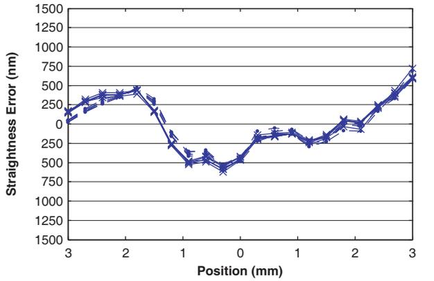
*ANT130V-5-PLUS straightness error; five runs, bi-directional, parallel to the wedge.*
