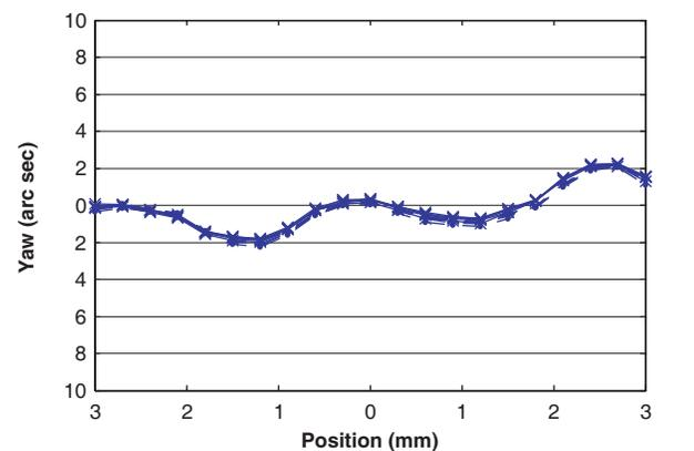
*ANT130V-5-PLUS yaw, five runs, bi-directional. Highly repeatable, minimal yaw error enhances system positioning accuracy.*
