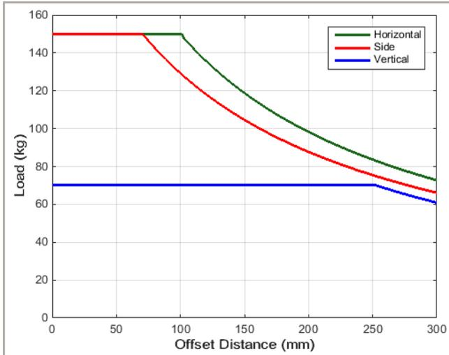
Cantilevered load capability of the PRO280SL/SLE.
