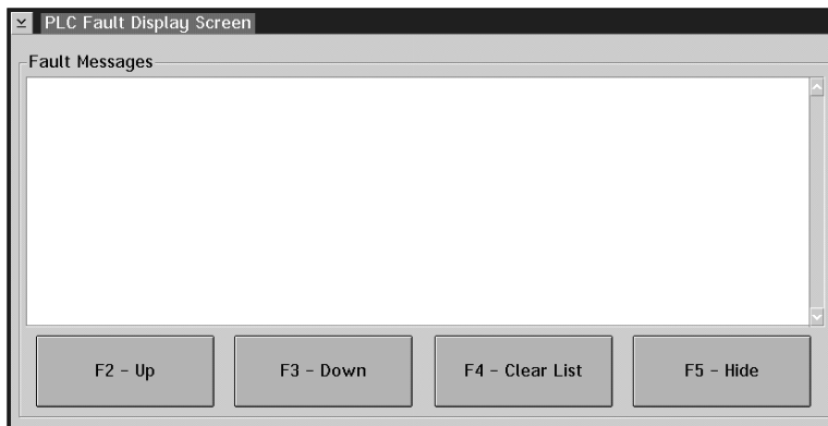
Figure 6-19. Fault Display Screen
