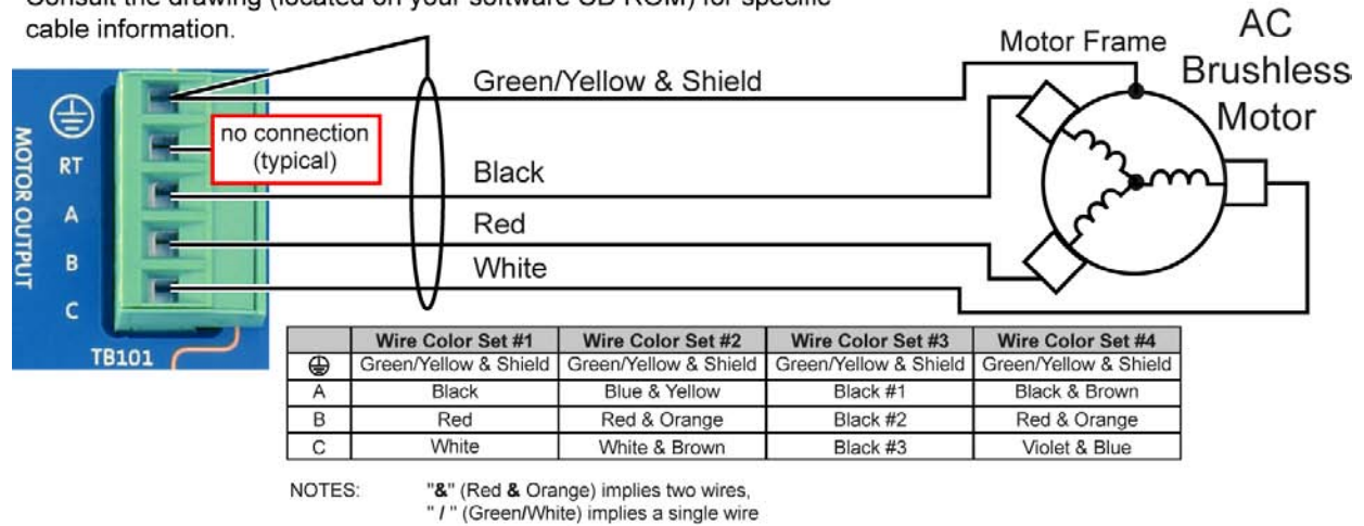
Figure 2-7. Brushless Motor Configuration
