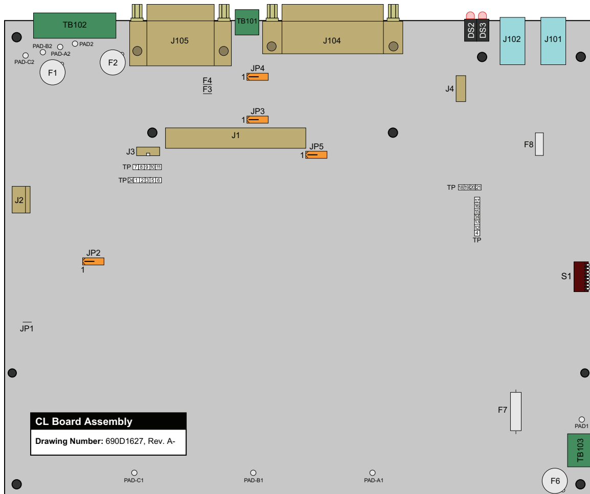
Figure 5-1: Control Board Assembly
