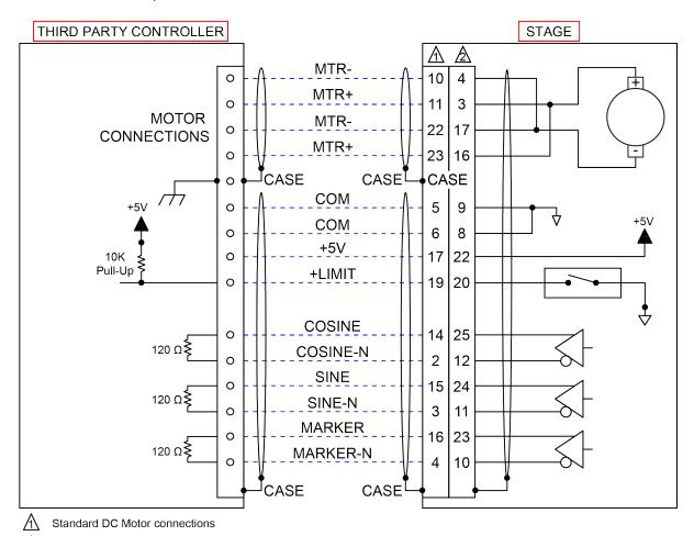
Figure 3-1: Motor and Feedback Wiring (-M1 Option)
