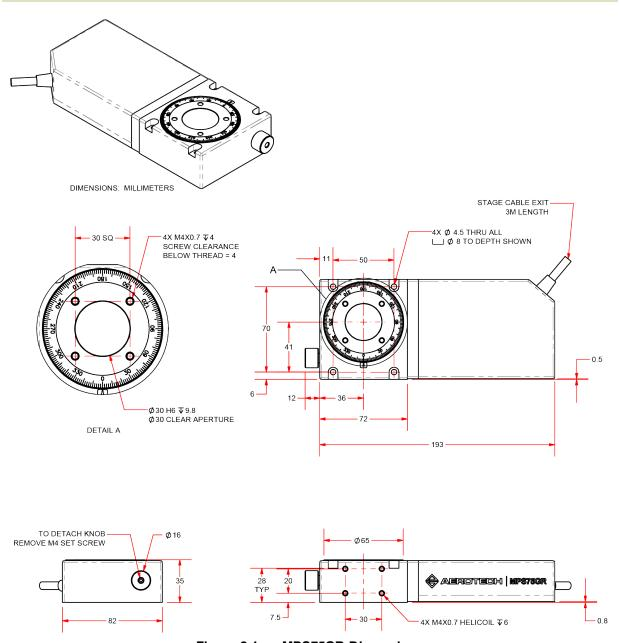
Figure 2-1: MPS75GR Dimensions
