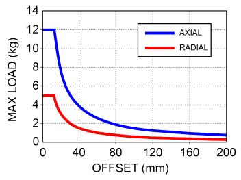
Figure 2-7: Load Capability of MPS75GR Series Stages
