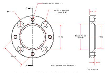
Figure 2-3: MPS75GR LMO Option Dimensions
