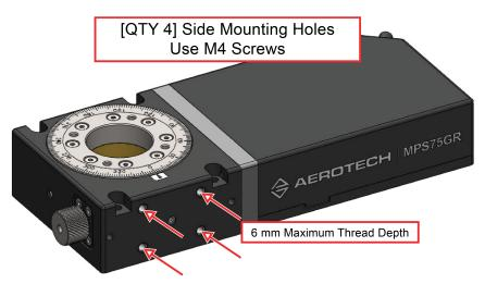
Figure 2-5: Side Mounting Holes
