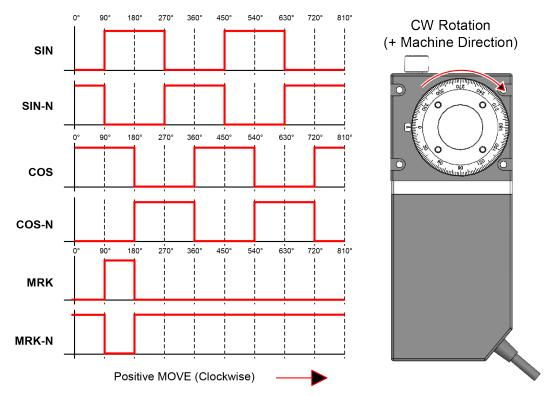
Figure 3-4: Encoder Phasing Reference Diagram (-M1 Option)
