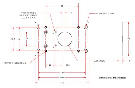
Figure 2-2: MPS75GR Mounting Plate Dimensions
