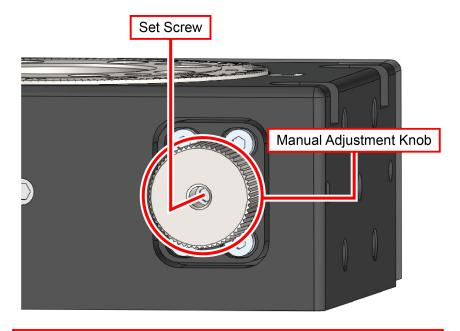
Remove Set Screw before attempting to remove the Manual Adjustment Knob
