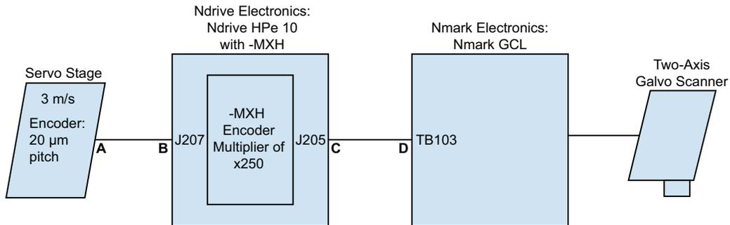
**Figure 4-1: Encoder Channel Signal Moves from the Servo Stage to the Nmark GCL**
