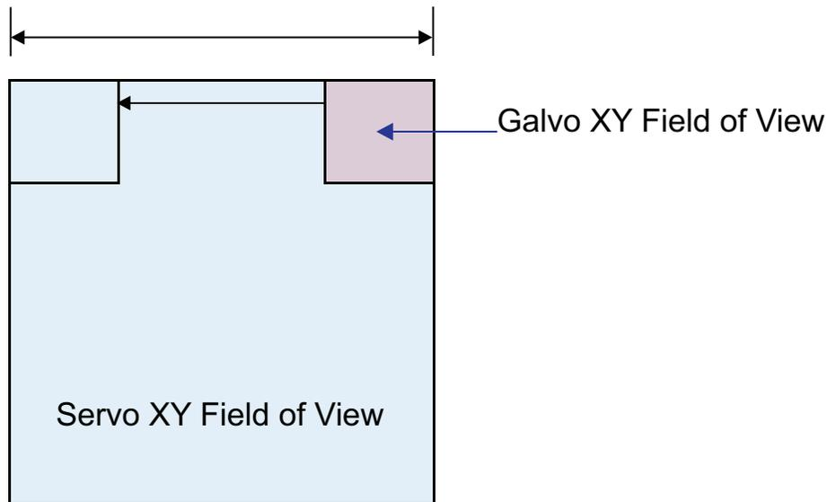
**Figure 1-3: Combined Galvo and Servo Fields of View**
