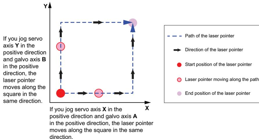
**Figure 3-1: Positive Motion Goes in the Same Direction**
