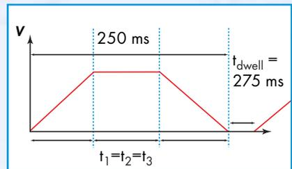
We now determine the peak speed required to make the move. In this case, because the move is symmetrical and divided into 3, the following formula is used:
