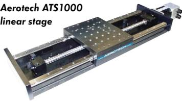
typically not precision-made and has inherent inaccuracies. The resulting high friction may minimize backlash but produces heat and wear, reducing accuracy and repeatability. The ball-screw system uses a ball nut on the screw and is therefore much more
