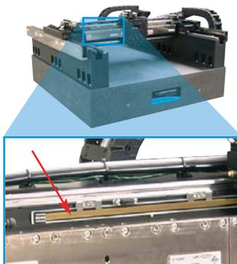
One of the major benefits of using a linear encoder system in a linear motor setup is that the reading head and scale can be placed very close to or at the bearing centerline, where it will measure the linear position at its most accurate point – i.e., free from Abbe errors that are caused by very small angular deviations in straightness and flatness being amplified by the distance between the bearing and the point of measurement.
