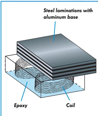
Due to the iron laminations in the forcer, an attractive force is now present between the forcer and the track and is proportional to the force produced by the motor. As a result of the laminations, a cogging force is now present on the motor. Care must also be taken when presenting the
