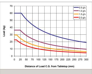
Pitch offsets with varying C.O.G. height and laterally centered payload.
