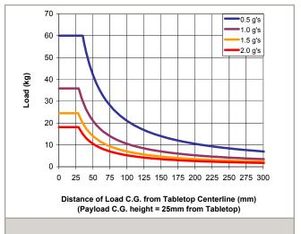
Yaw offsets with payload C.O.G. 25 mm above the tabletop.
