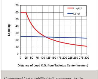
Cantilevered load capability (static conditions) for the ABL1500WB.
