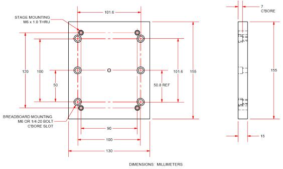
Figure 2-3: ANT130V-5 Mounting Plate (-MP) Dimensions
