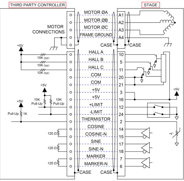
Figure 3-2: Motor and Feedback Wiring [-CN2 option]
