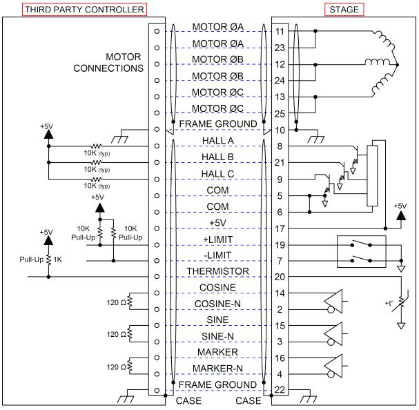
Figure 3-1: Motor and Feedback Wiring [-CN1 option]
