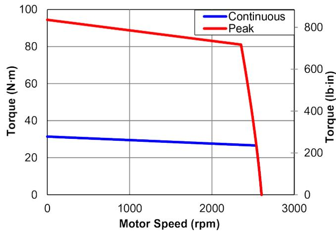
Figure 1-11: BM4500 Torque Speed Curves
