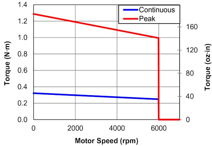
Figure 1-13: BMS60 Torque Speed Curves
