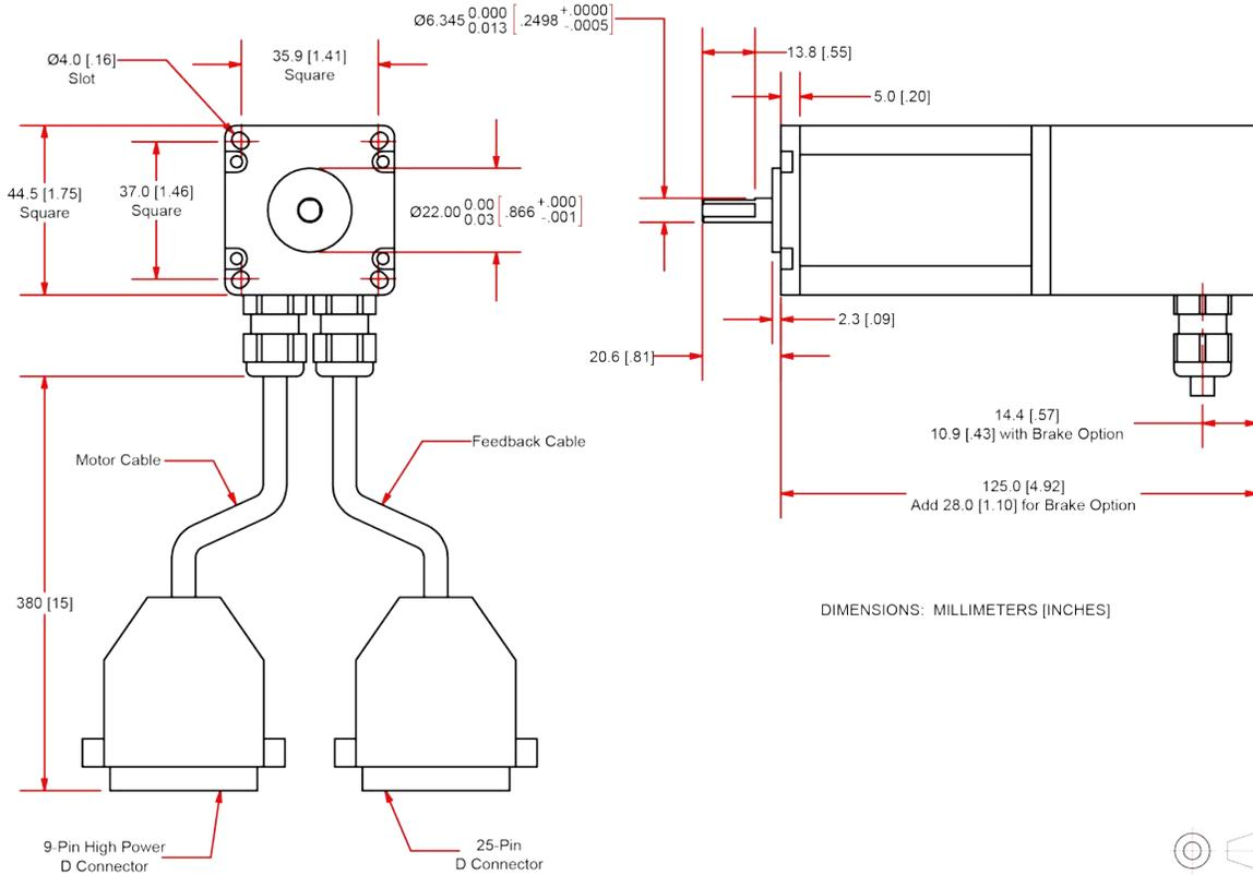
Figure 1-22: BMS35 Model Dimensions (NEMA 17)
