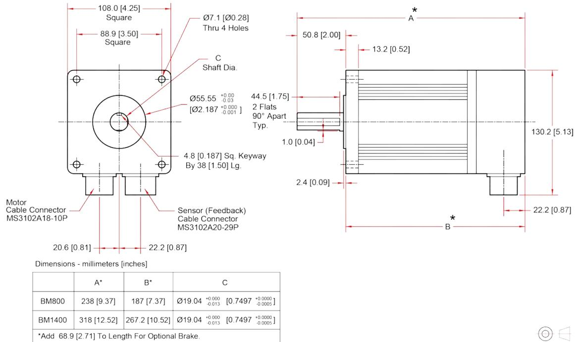
Figure 1-20: BM800, BM1400 Model Dimensions (NEMA 42)
