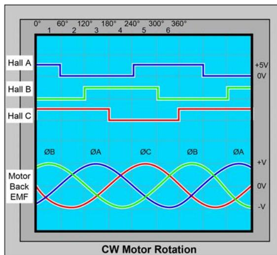
During CW rotation, each Hall effect signal is at a logic high state when its corresponding motor phase is at a negative voltage.
