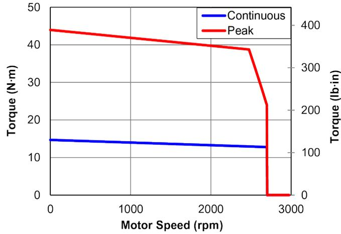
Figure 1-9: BM2000 Torque Speed Curves
