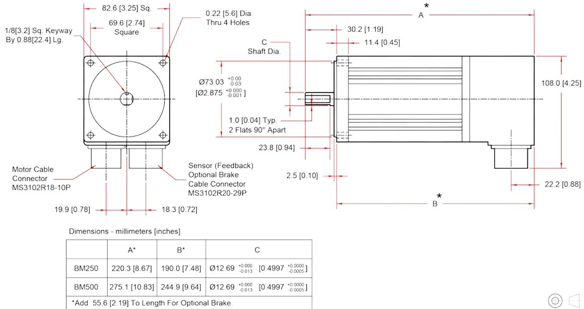
Figure 1-19: BM250, BM500 Model Dimensions (NEMA 34)
