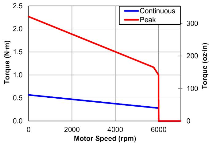
Figure 1-14: BMS100 Torque Speed Curves
