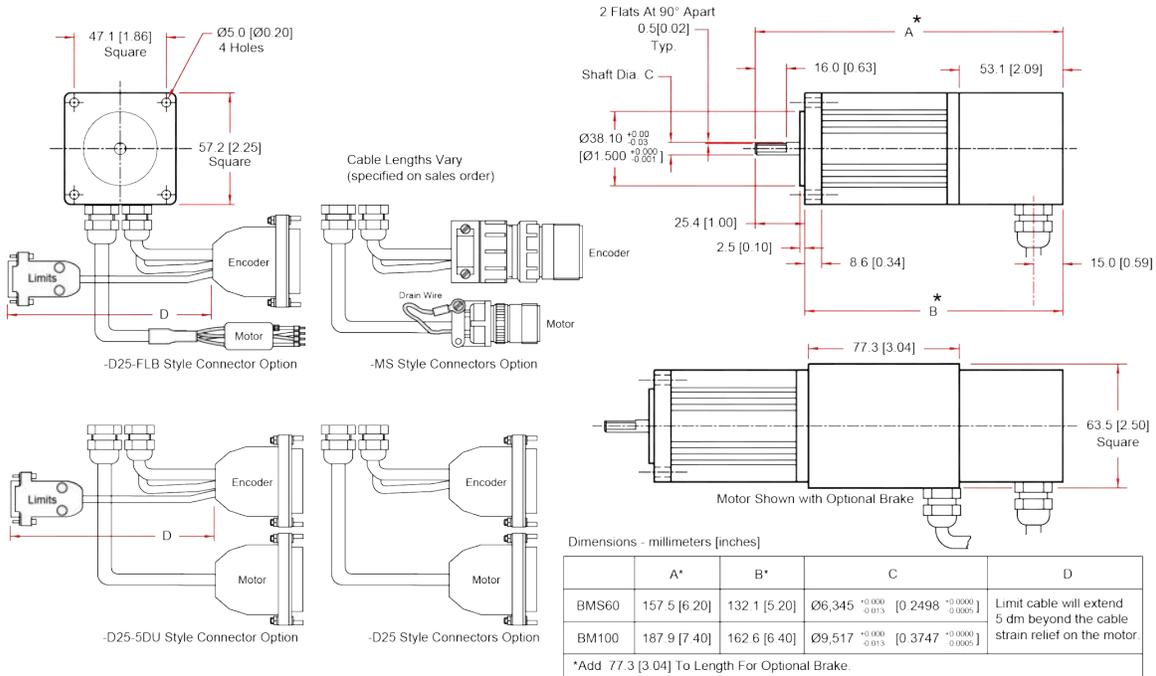
Figure 1-23: BMS60 and BMS100 Model Dimensions (NEMA 23)
