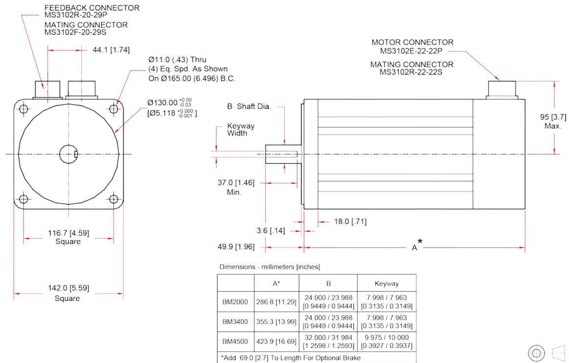
Figure 1-21: BM2000, BM3400, BM4500 Model Dimensions (NEMA 56)
