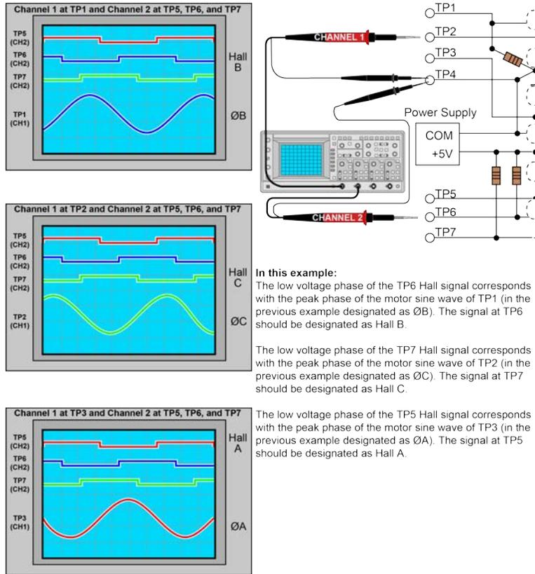
Figure 2-6: Hall Phasing with Oscilloscope
