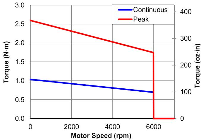
Figure 1-3: BM130 Torque Speed Curves
