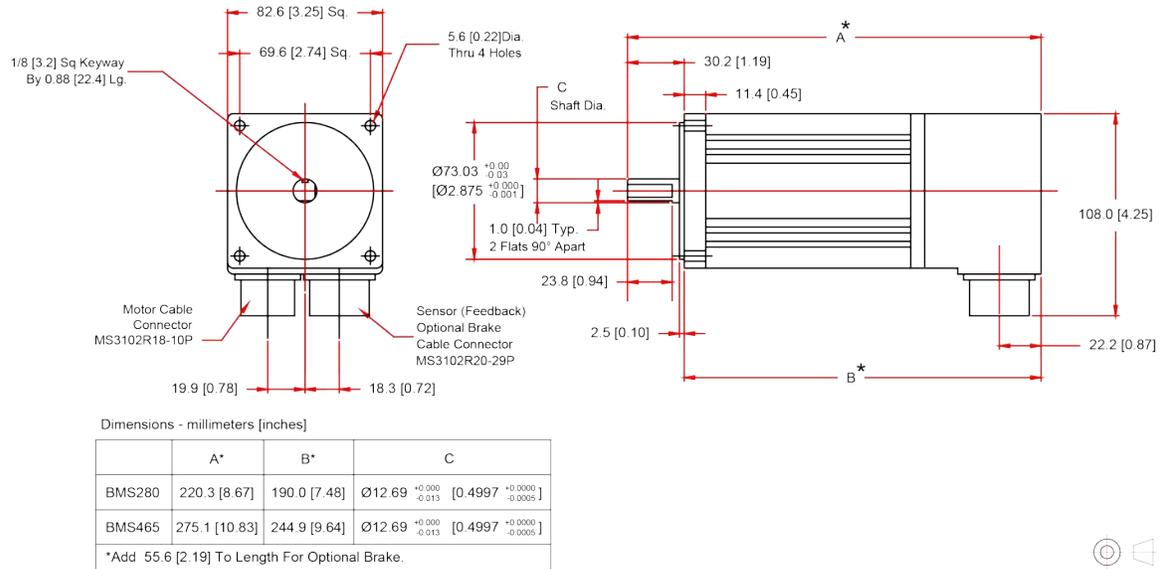
**Figure 1-24: BMS280 and BMS465 Model Dimensions (NEMA 34)**
