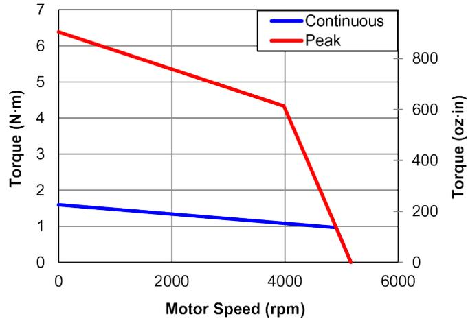
Figure 1-15: BMS280 Torque Speed Curves
