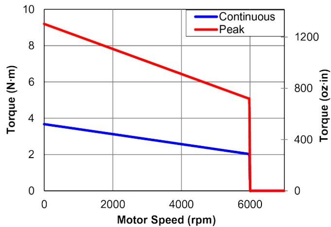
Figure 1-6: BM500 Torque Speed Curves
