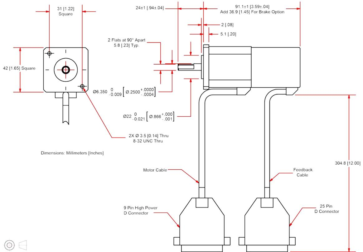
**Figure 1-17: BM22 Model Dimensions (NEMA 17)**
