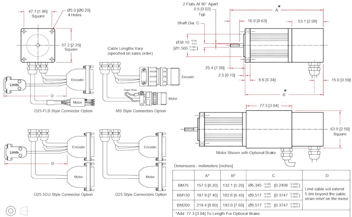
Figure 1-18: BM75, BM130, BM200 Model Dimensions (NEMA 23)
