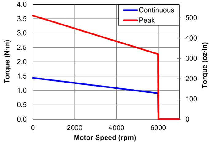
Figure 1-4: BM200 Torque Speed Curves
