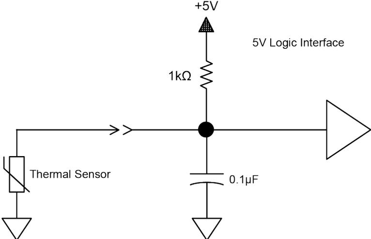
**Figure 2-2: Typical Thermistor Interface Circuit**
