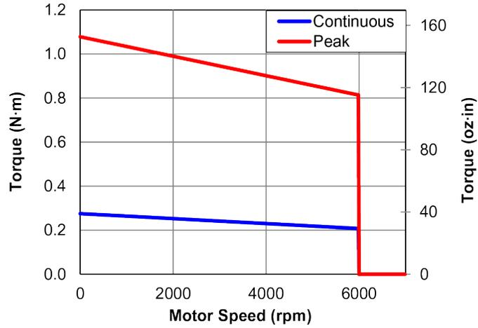
Figure 1-12: BMS35 Torque Speed Curves
