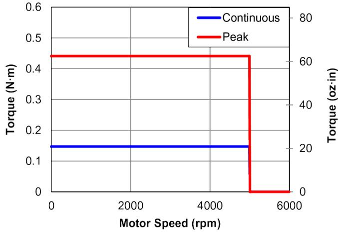
Figure 1-1: BM22 Torque Speed Curves
