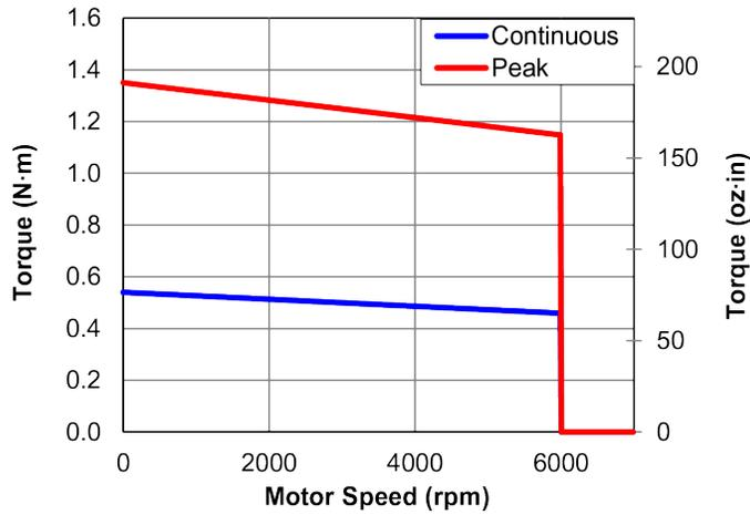
Figure 1-2: BM75 Torque Speed Curves
