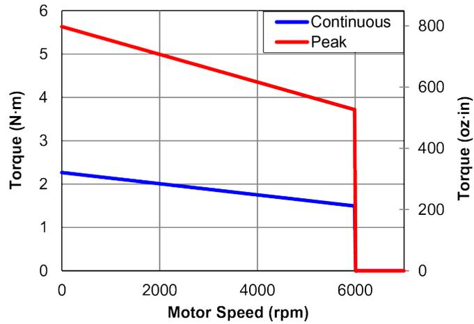
Figure 1-5: BM250 Torque Speed Curves
