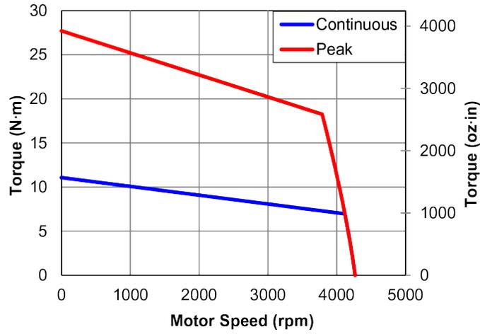
Figure 1-8: BM1400 Torque Speed Curves
