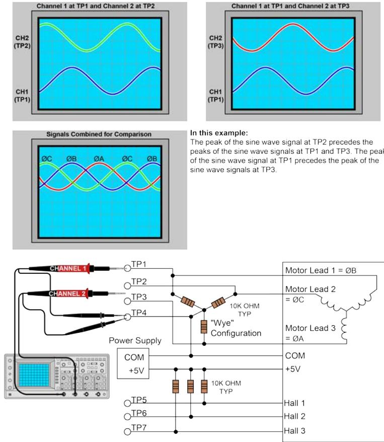
**Figure 2-5: Motor Lead Phasing with Oscilloscope**
