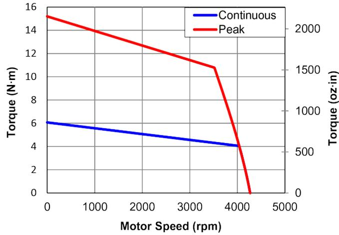
Figure 1-7: BM800 Torque Speed Curves
