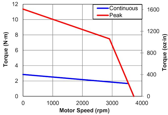
Figure 1-16: BMS465 Torque Speed Curves
