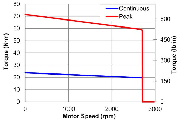
Figure 1-10: BM3400 Torque Speed Curves
