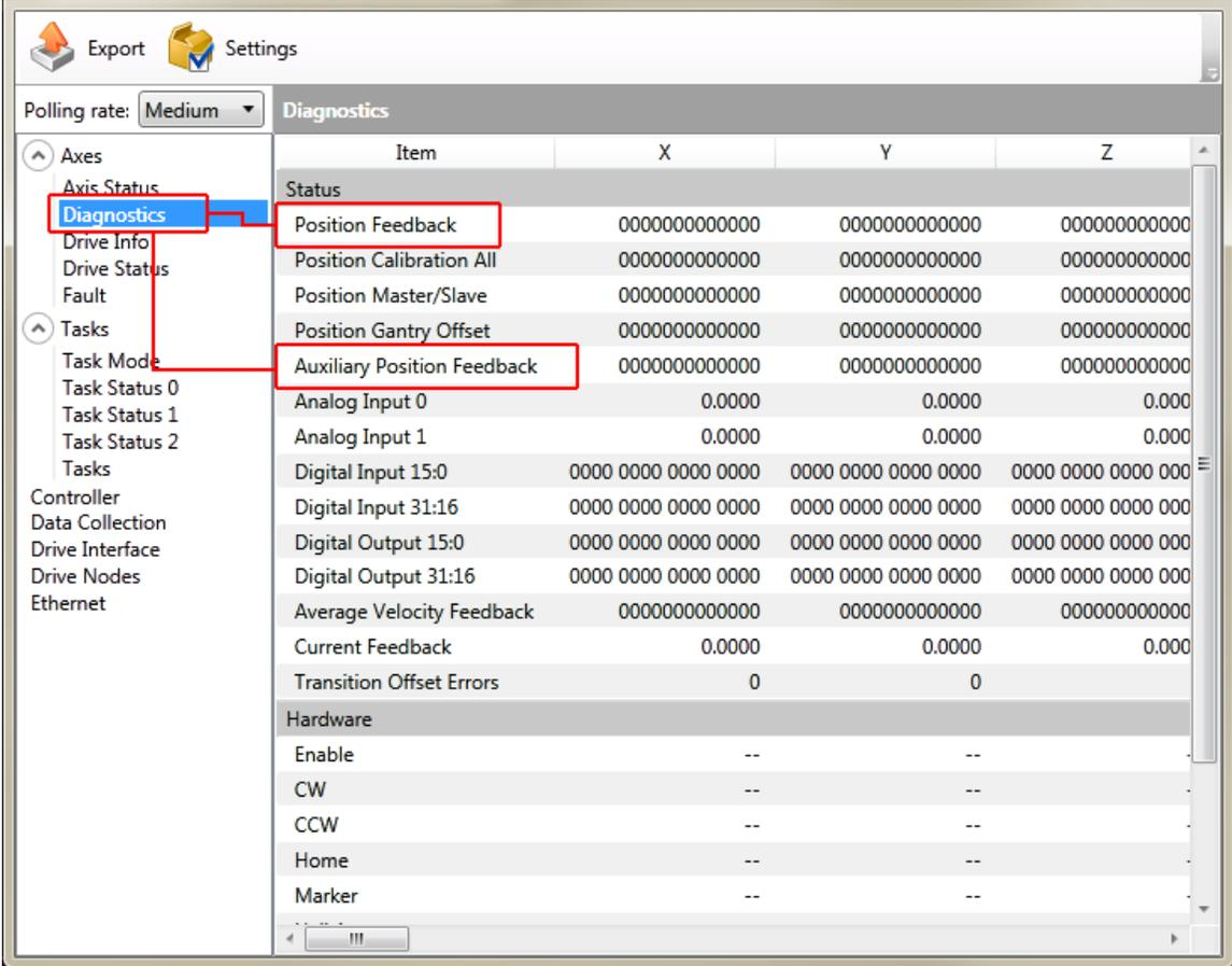
Figure 2-19: Position Feedback in the Diagnostic Display
