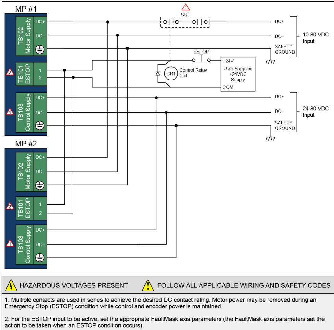
**Figure 2-28: Typical Emergency Stop Circuit**
