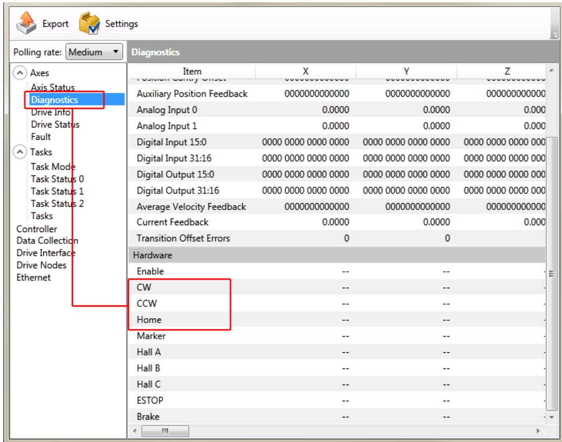
**Figure 2-25: Limit Input Diagnostic Display**
