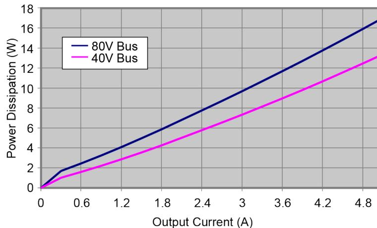
Figure 1-3: Power Dissipation vs. Output Current
