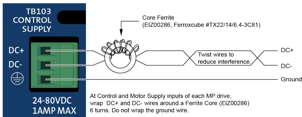
Figure 2-1: Control Supply Connections
