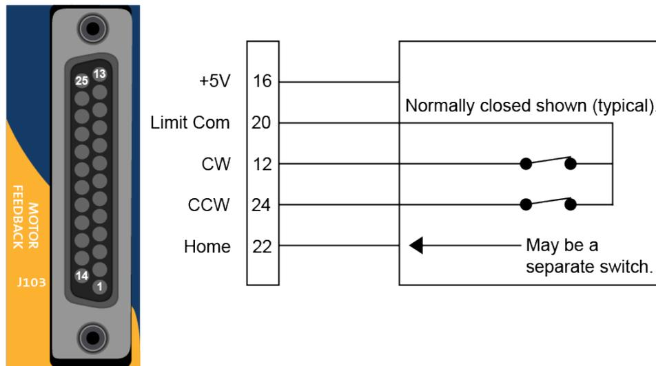
Figure 2-23: End of Travel Limit Input Connections
