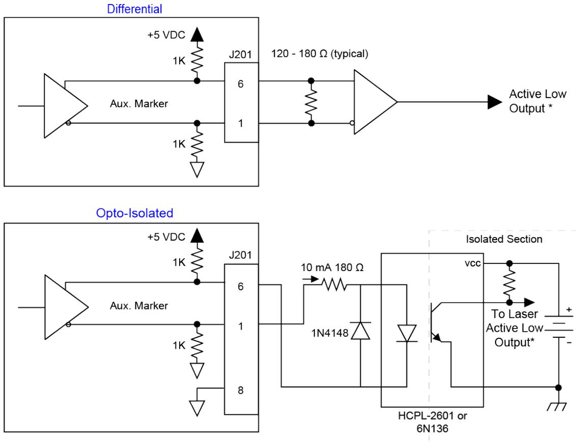
\* Active low output shown. Opposite polarity available by reversing connections to Pins 1 and 6.
