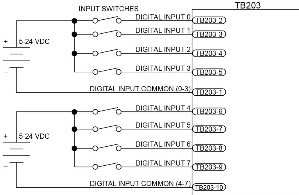
Figure 3-10: Digital Inputs Connected to a Current Sourcing Device
