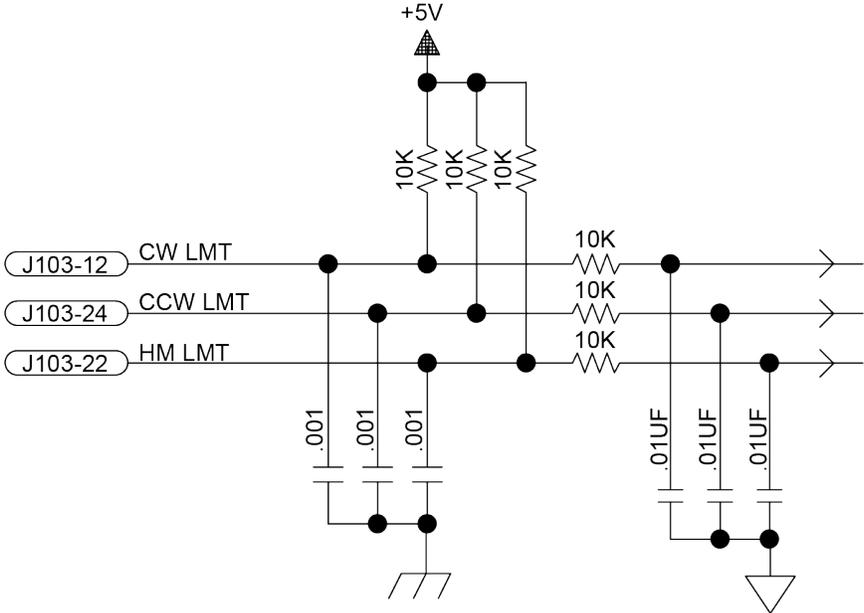
Figure 2-24: End of Travel Limit Interface Input (J103)
