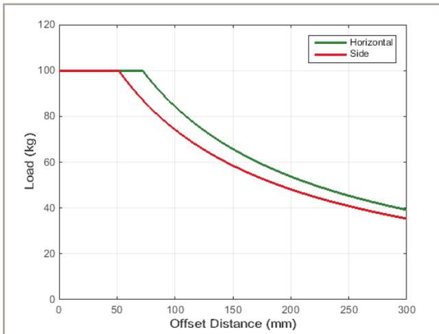
*Cantilevered load capability of the PRO225LM.*
