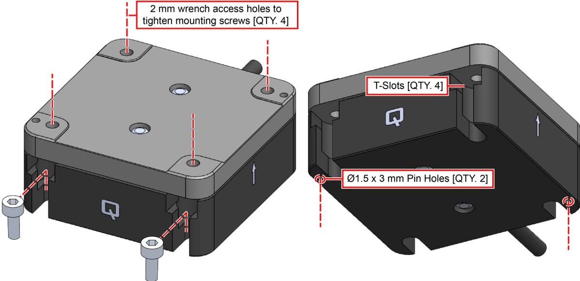
Figure 2-4: Mounting Hole Locations
