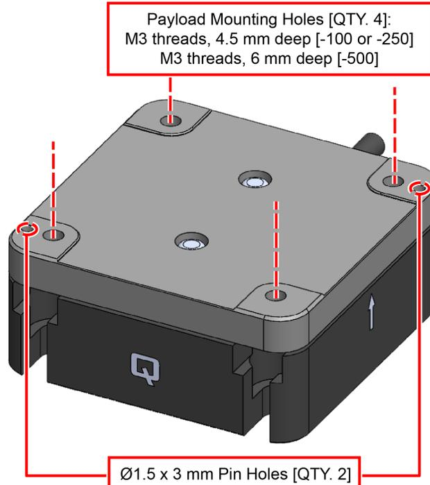
**Figure 2-5: Mounting Hole Locations (Tabletop)**
