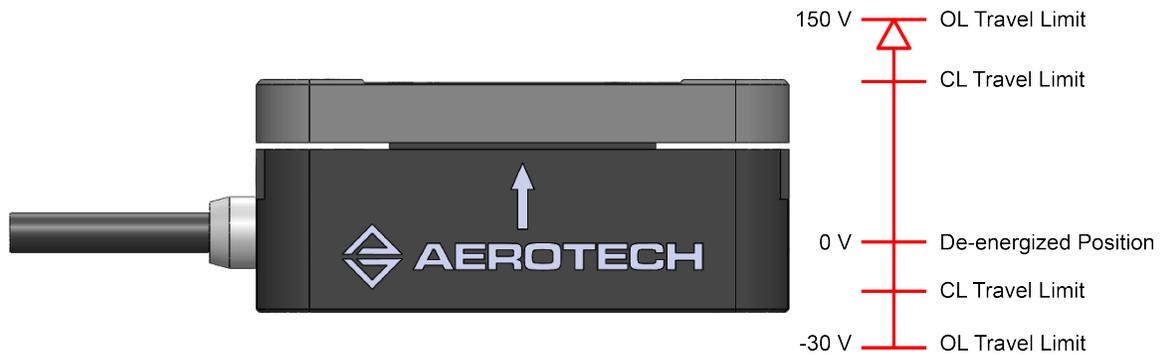
**Figure 1-1: Single-Axis Stage Travel and Voltage Relationship**
