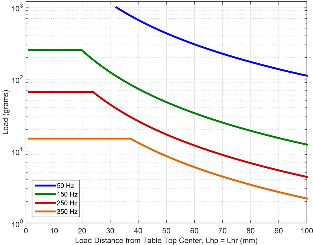
Figure 2-10: QNP50Z-250, 1st Natural Frequencies for Point Load Offset from Tabletop Center in HP Direction
