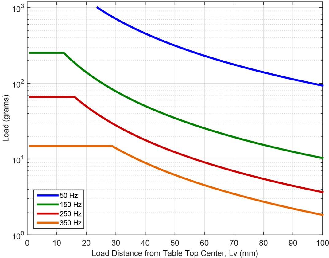
Figure 2-12: QNP50Z-250, 1st Natural Frequencies for Point Load Offset from Tabletop Center in V Direction
