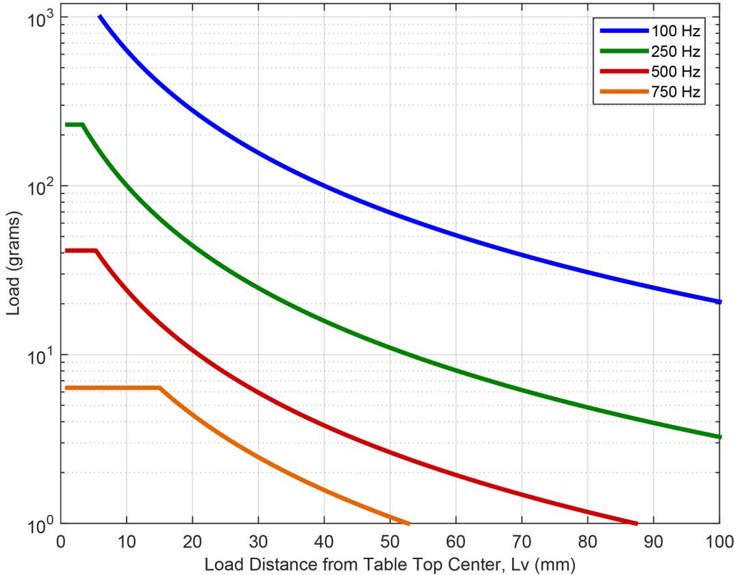
Figure 2-9: QNP40Z-100, 1st Natural Frequencies for Point Load Offset from Tabletop Center in V Direction
