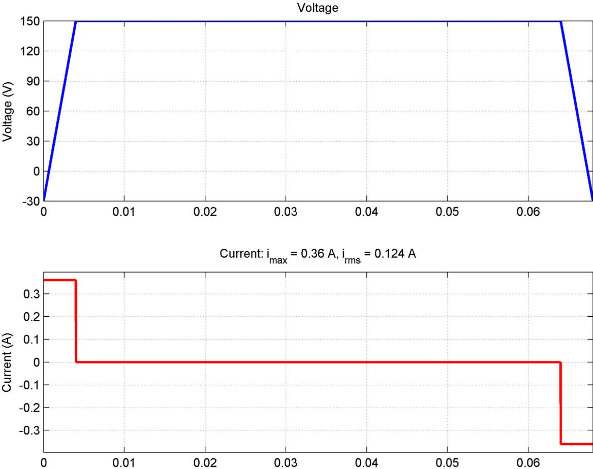
Figure C-12: Voltage and current waveforms for the profile commanded in Example 2
