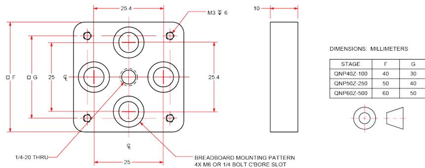
**Figure 2-2: Mounting Plate (-MP) Dimensions**
