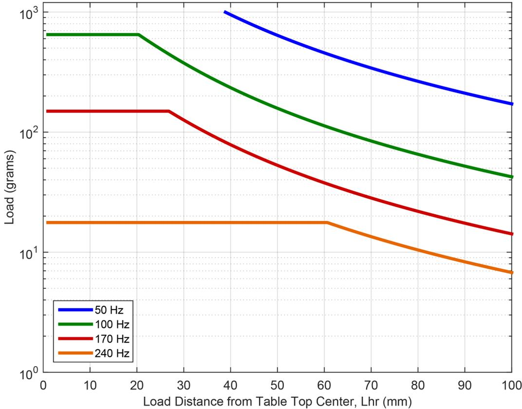
Figure 2-14: QNP60Z-500, 1st Natural Frequencies for Point Load Offset from Tabletop Center in HR Direction
