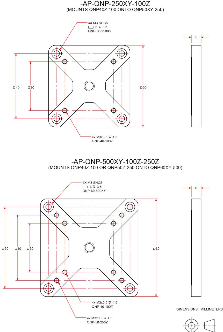
**Figure 2-3: Adapter Plate (-AP) Dimensions**
