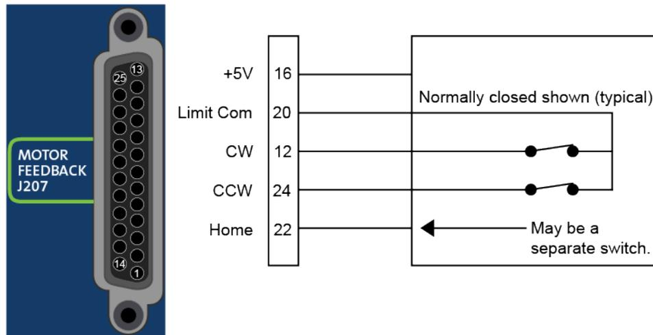
Figure 2-20: End of Travel Limit Input Connections
