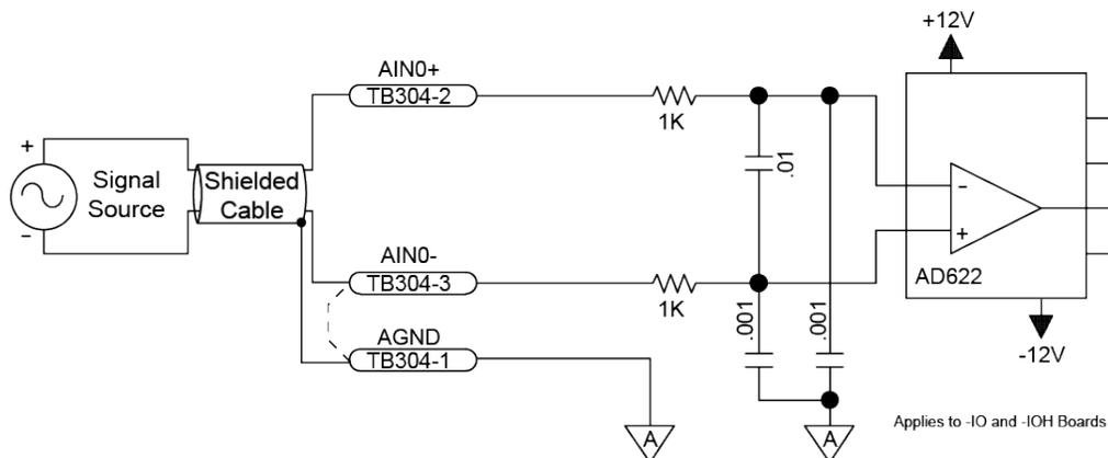
**Figure 3-7: Analog Input Typical Connection (TB304)**
