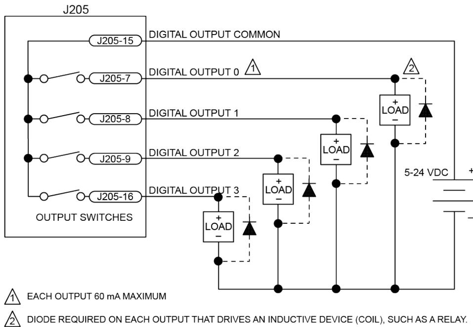
**Figure 2-27: Outputs Connected in Current Sourcing Mode (J205)**
