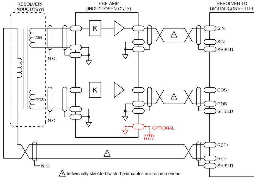
**Figure 4-2: Resolver/Inductosyn Recommended Wiring**
