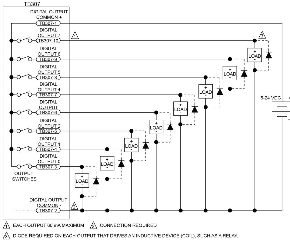
**Figure 3-12: Digital Outputs Connected in Current Sourcing Mode**
