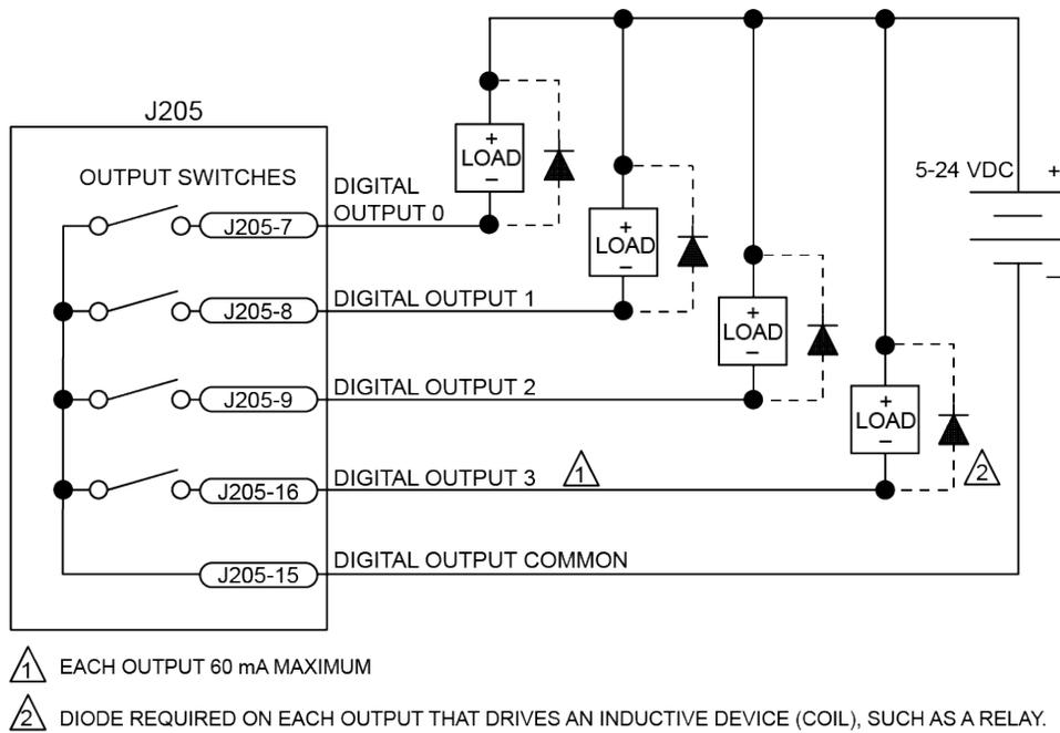
**Figure 2-28: Outputs Connected in Current Sinking Mode (J205)**
