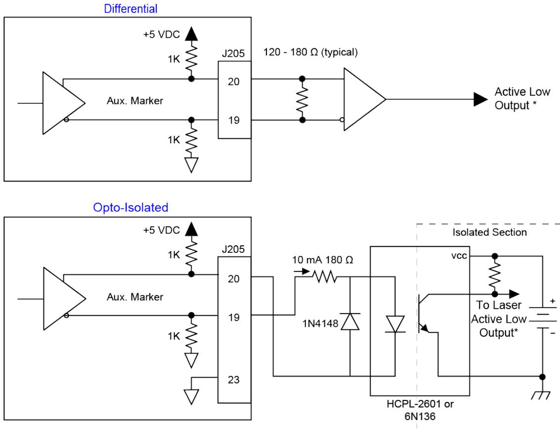
\* Active low output shown. Opposite polarity available by reversing connections to Pins 19 and 20.
