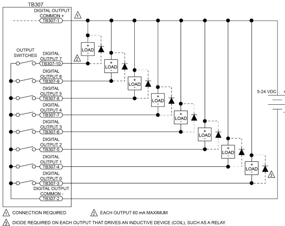
**Figure 3-13: Digital Outputs Connected in Current Sinking Mode**
