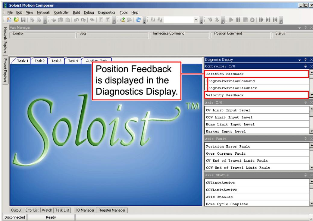
Figure 2-16: Position Feedback in the Diagnostic Display
