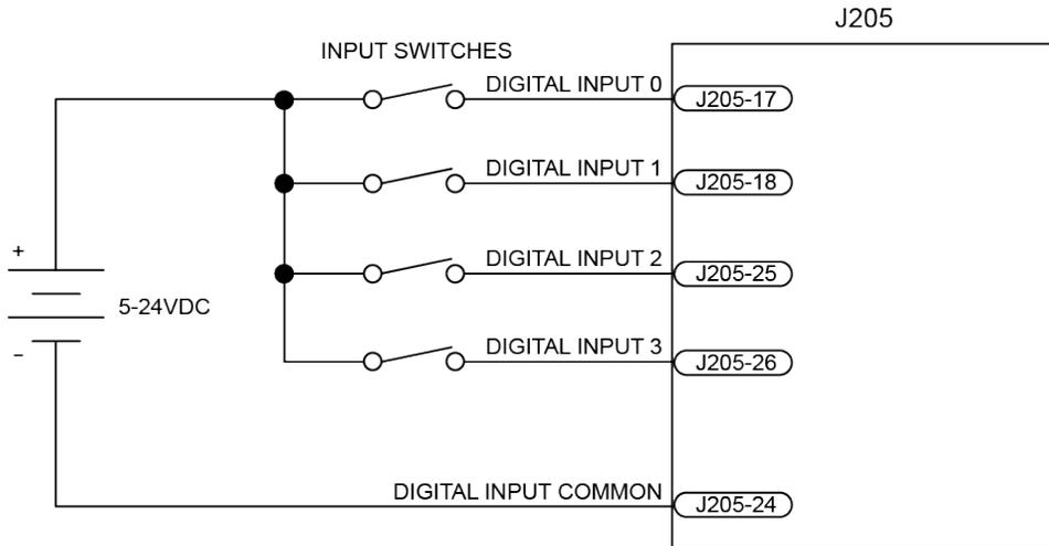
**Figure 2-29: Inputs Connected in Current Sourcing Mode (J205)**
