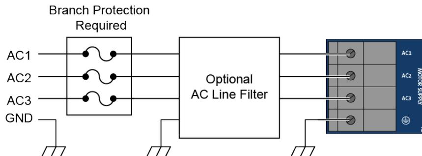
**Figure 2-2: Motor Bus Input Connections**
