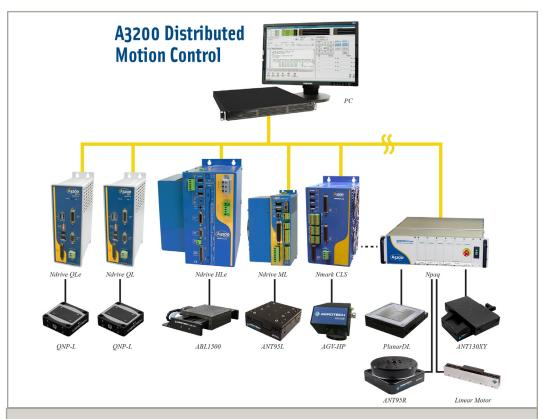
The Ndrive QL and Ndrive QLe enables coordinated motion of piezo axes and brushless, DC brush, and stepper motor axes with the powerful A3200 software-based motion control platform.
