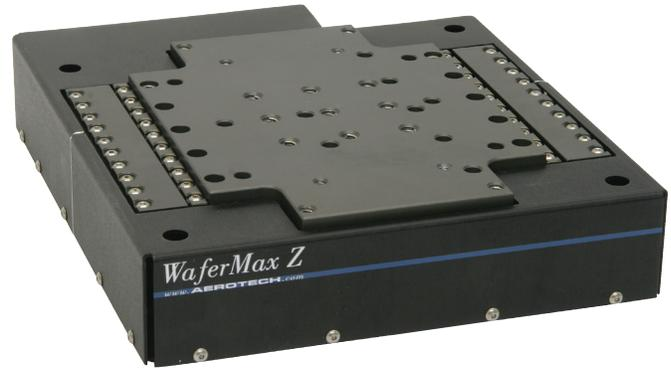
The WaferMaxZ represents a significant breakthrough in vertical alignment of high-precision components in one compact package. Its superior noncontact linear motor drive employs a high-accuracy encoder for direct position feedback. When combined with Aerotech's MXH multiplier, it offers sub-nanometer resolution in addition to high speed and accuracy.
