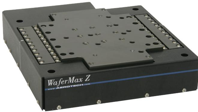
The WaferMaxZ represents a significant breakthrough in vertical alignment of high-precision components in one compact package. Its superior noncontact linear motor drive employs a high-accuracy encoder for direct position feedback. When combined with Aerotech's MXH multiplier, it offers sub-nanometer resolution in addition to high speed and accuracy.
