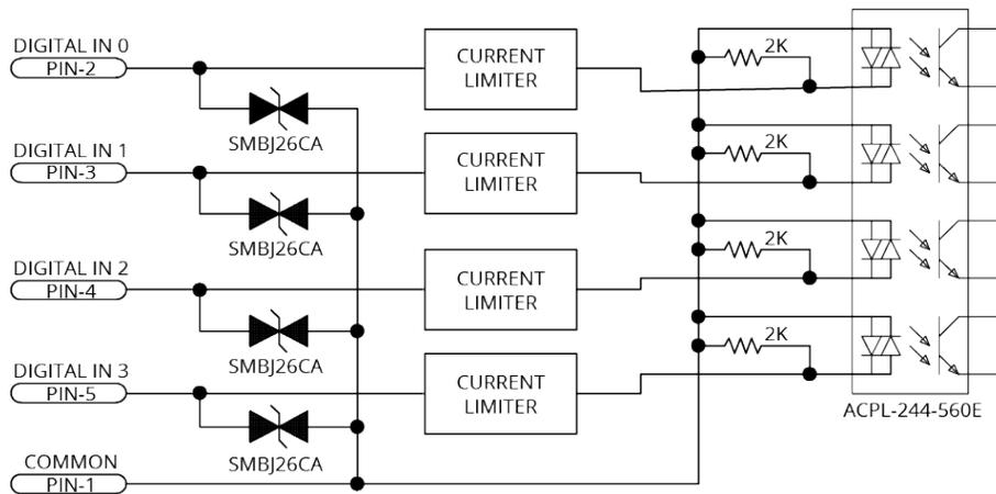
**Figure 3-8: Digital Inputs Schematic [-EB1]**
