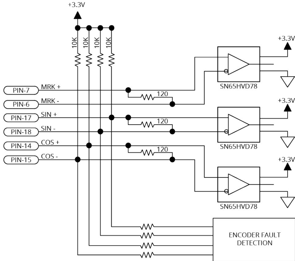
**Figure 2-12: Square Wave Encoder Schematic (Feedback Connector)**
