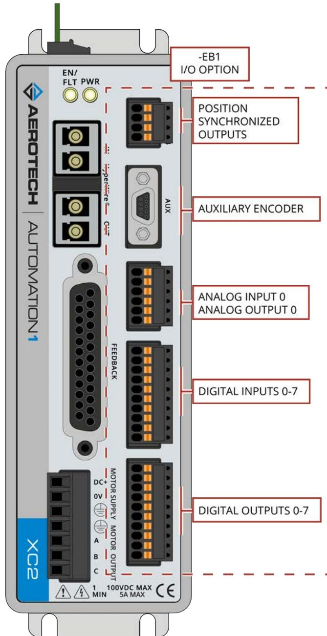
Figure 3-1: XC2 with -EB1 I/O Option Board Connectors
