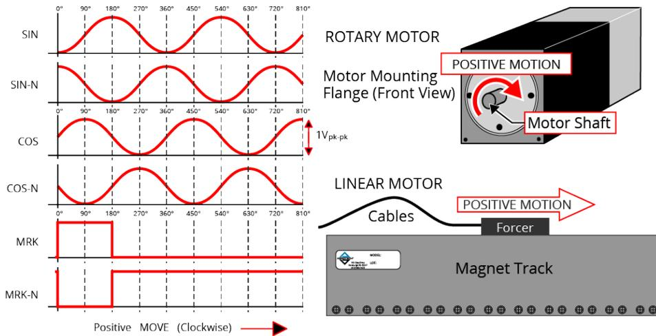
**Figure 2-14: Sine Wave Encoder Phasing Reference Diagram**
