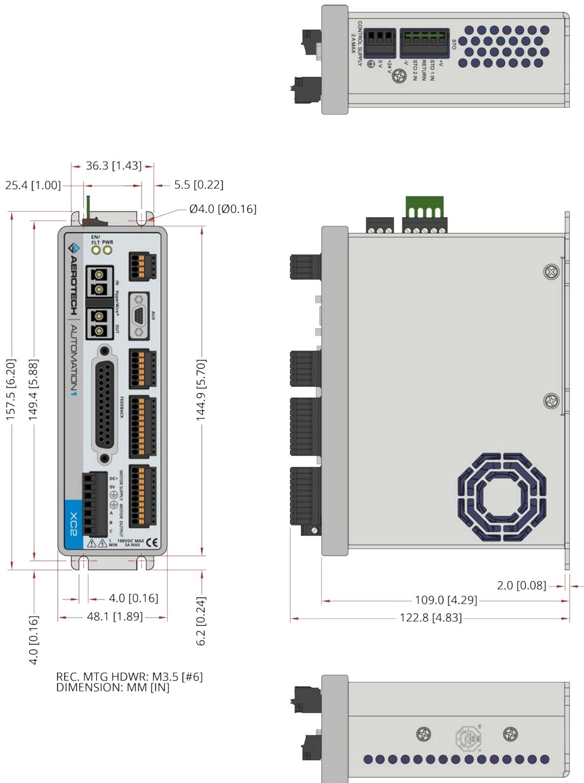
Figure 1-4: Dimensions [-EB1]
