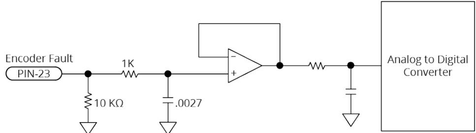
**Figure 2-20: Encoder Fault Input Schematic (Feedback Connector)**
