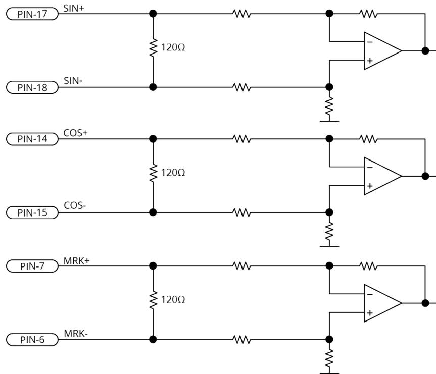
**Figure 2-22: Sine Wave Encoder Schematic (Feedback Connector)**
