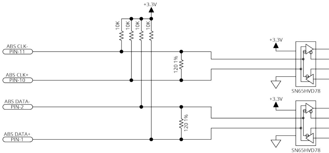
**Figure 2-35: Absolute Encoder Schematic (Auxiliary I/O Connector)**
