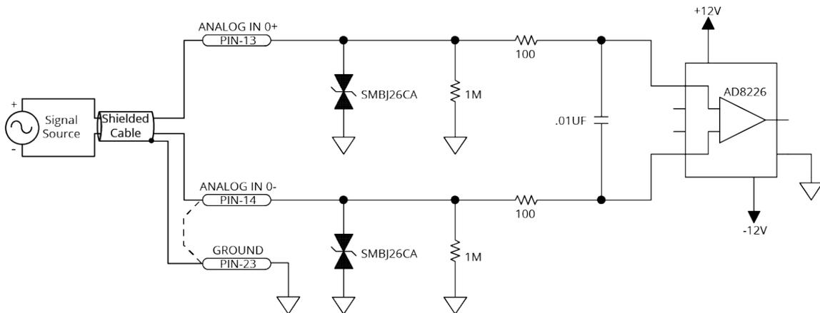
**Figure 2-47: Analog Input 0 Schematic**
