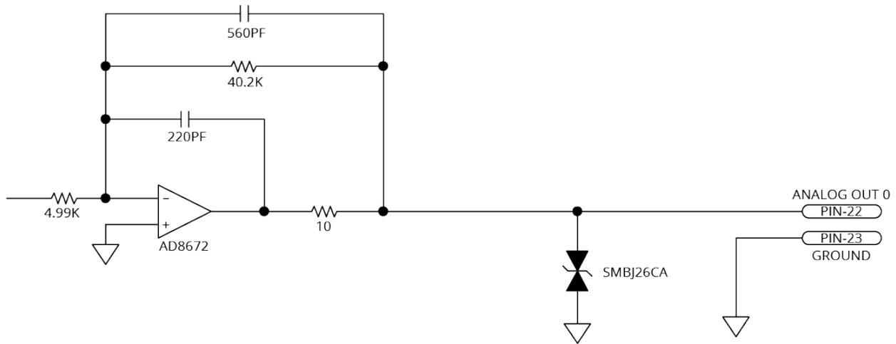
**Figure 2-46: Analog Output 0 Schematic**
