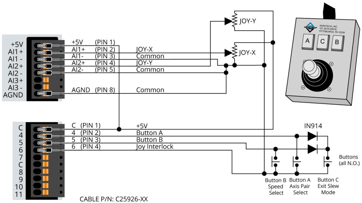
Figure 4-2: Two Axis Joystick Interface (to the I/O board)
