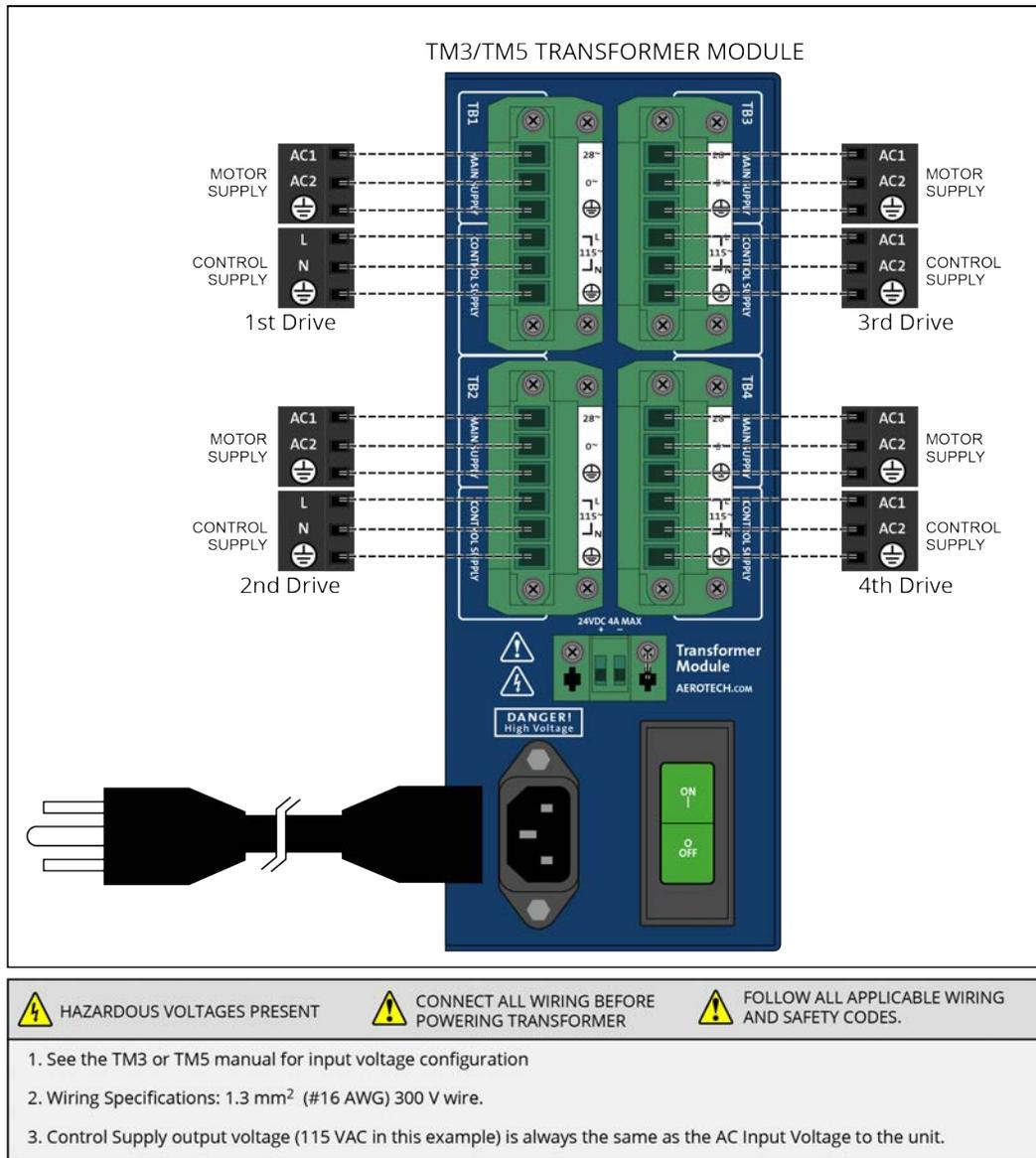
**Figure 2-9: TM3/TM5 Transformer Control and Motor Power Wiring**
