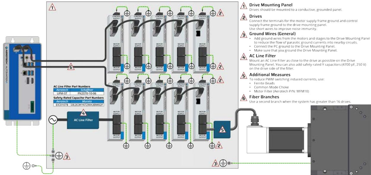
Figure 2-48: System Wiring Drawing (Best Practice)
