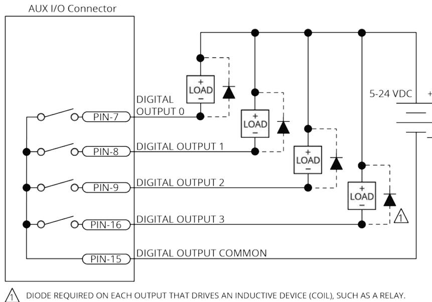
**Figure 2-41: Digital Outputs Connected in Current Sinking Mode**
