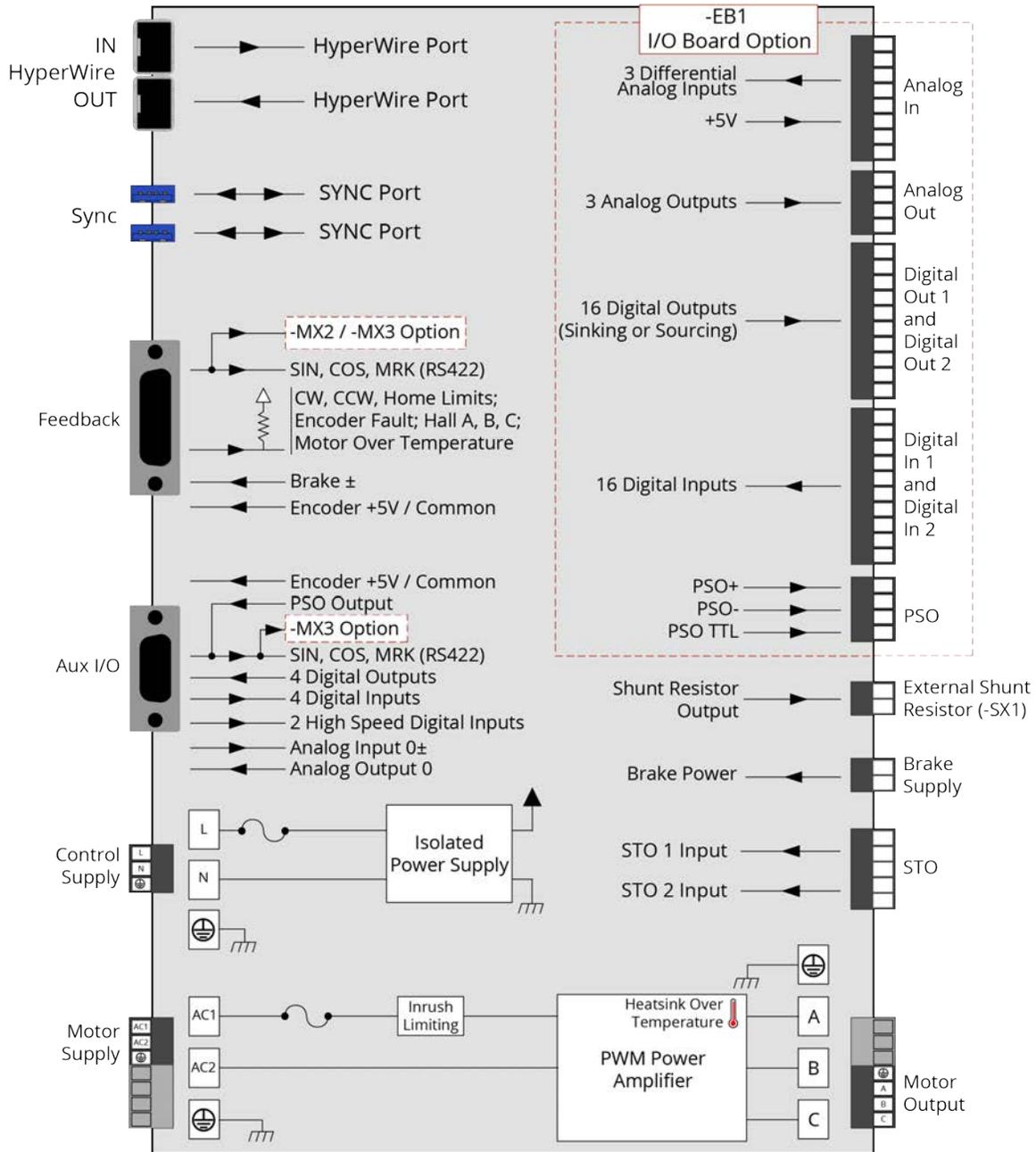
Figure 1-2: Functional Diagram
