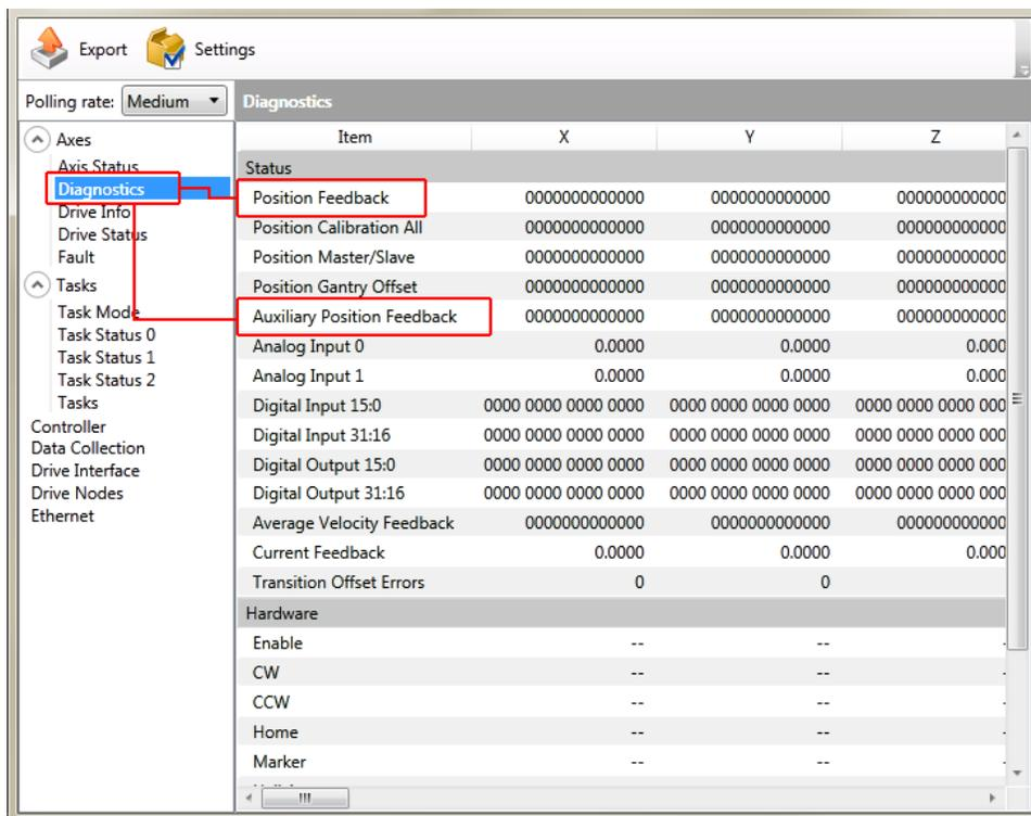
**Figure 2-24: Position Feedback in the Diagnostic Display**
