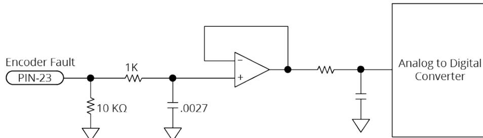
**Figure 2-27: Encoder Fault Input Schematic (Feedback Connector)**
