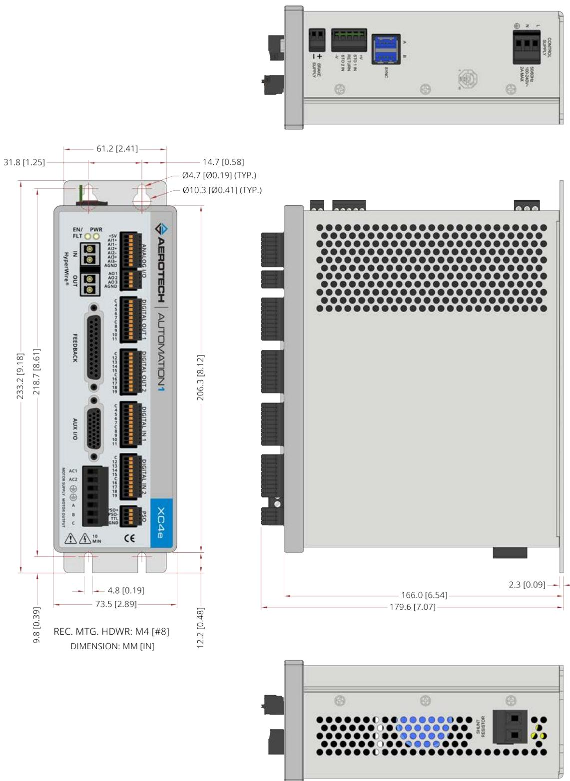
Figure 1-4: Dimensions [-EB1]
