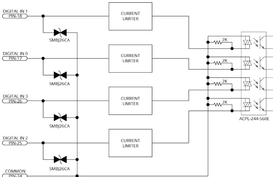
**Figure 2-42: Digital Inputs Schematic (Aux I/O Connector)**
