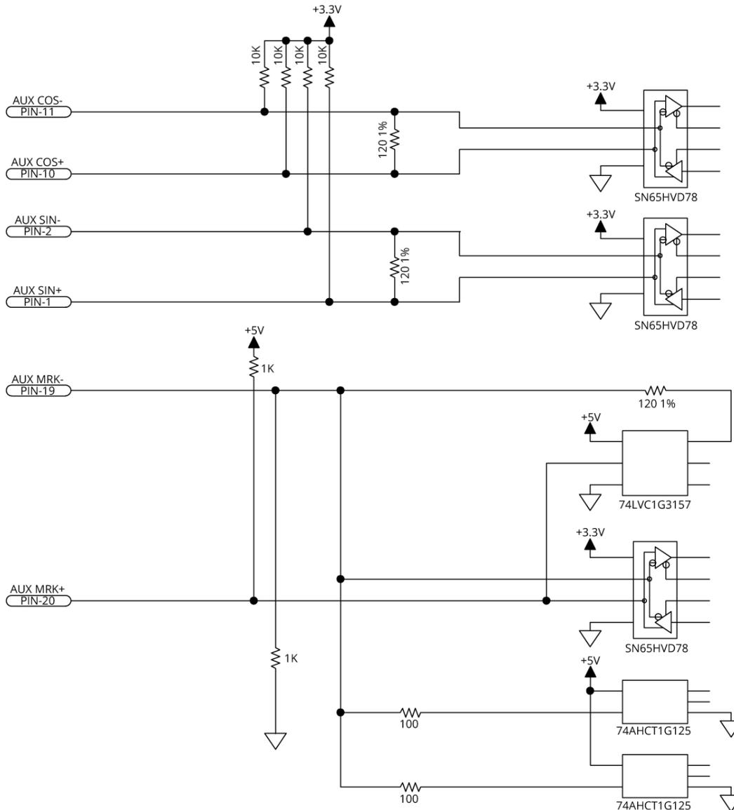
**Figure 2-34: Square Wave Encoder Interface (Aux I/O Connector)**
