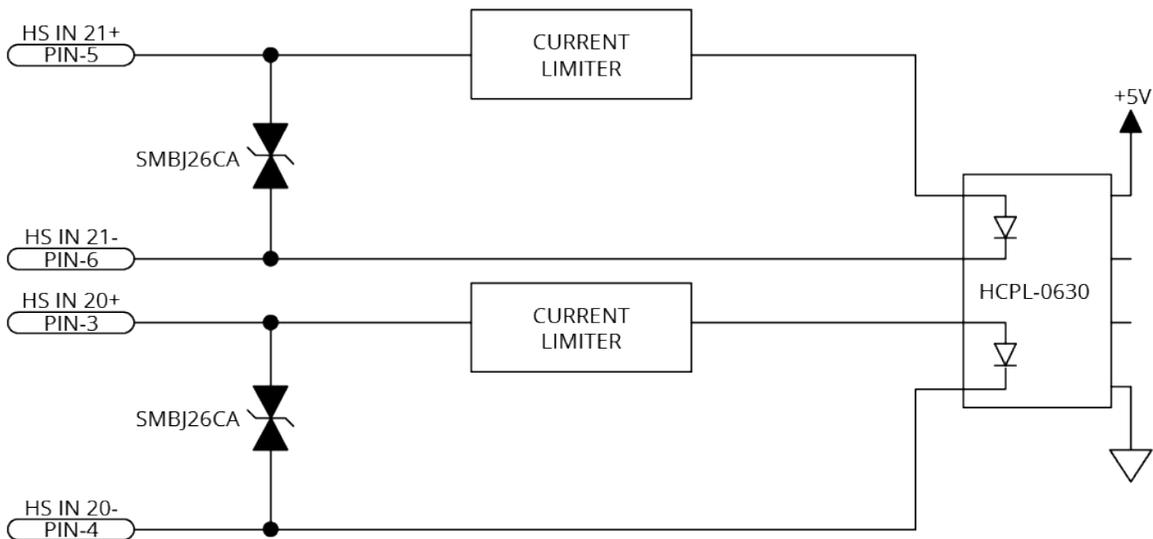
**Figure 2-45: High-Speed Inputs**
