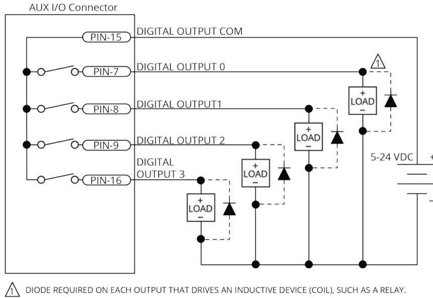
**Figure 2-40: Digital Outputs Connected in Current Sourcing Mode**
