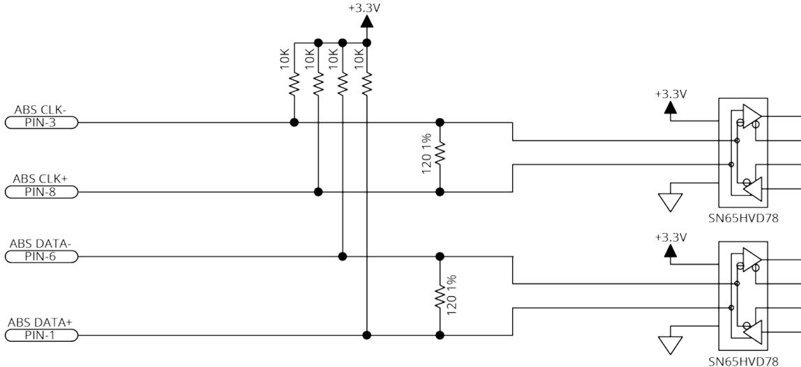
**Figure 2-37: Absolute Encoder Schematic (Aux Encoder Connector)**
