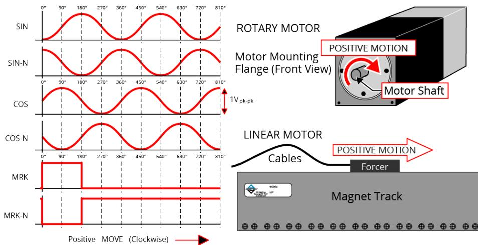
**Figure 2-38: Sine Wave Encoder Phasing Reference Diagram**
