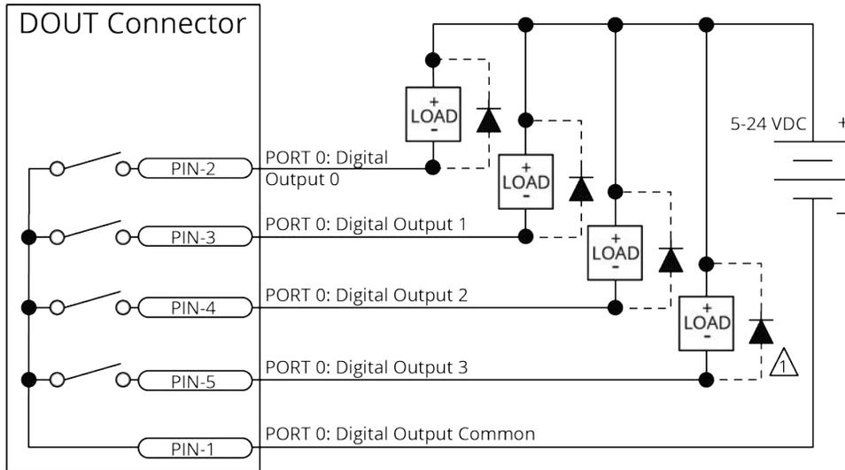
⚠ Diode required on each output that drives an inductive device (coil), such as a relay.
