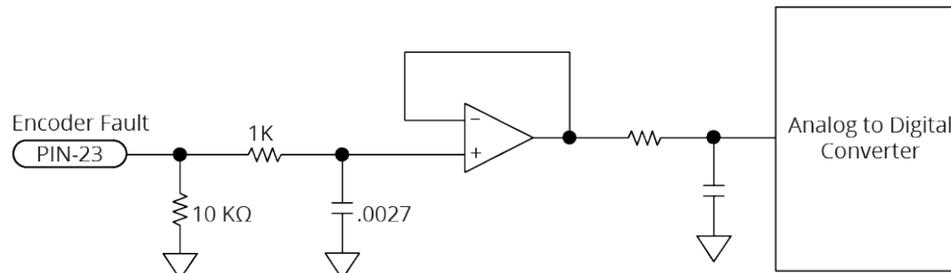
**Figure 2-19: Encoder Fault Input Schematic (Feedback Connector)**
