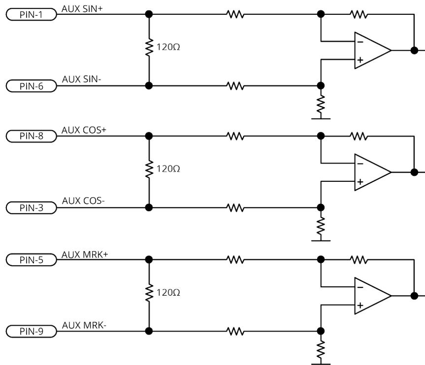
Figure 2-39: Sine Wave Encoder Schematic (Aux Encoder Connector)
