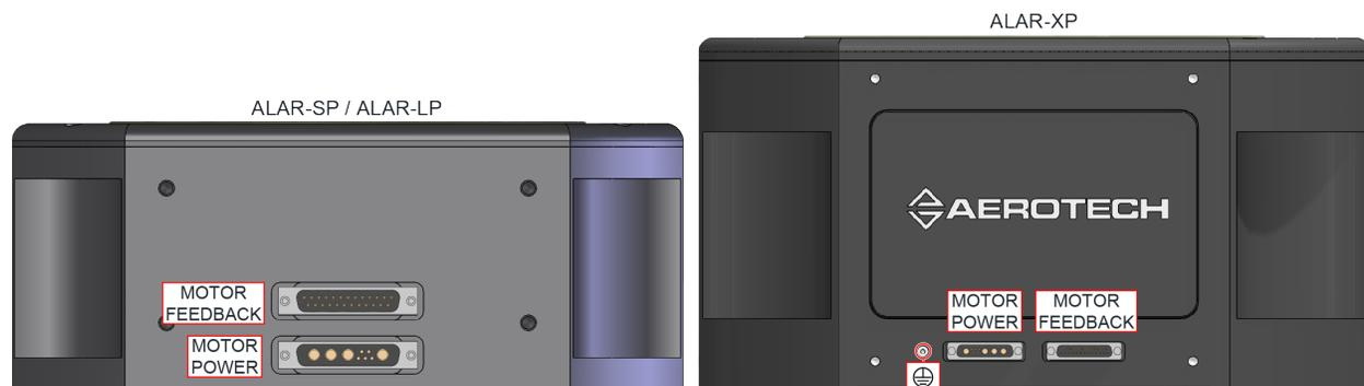
Figure 3-1: Electrical Connections
