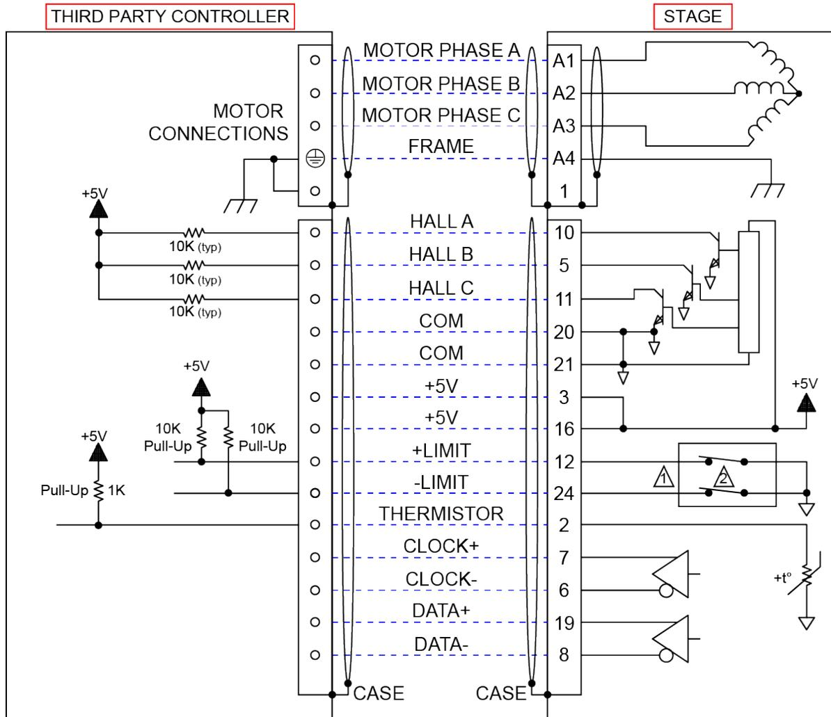
⚠ Over-Travel limit switches are present in -TRxxx option (Limited Travel) models only (continuous travel models do not have this feature).
