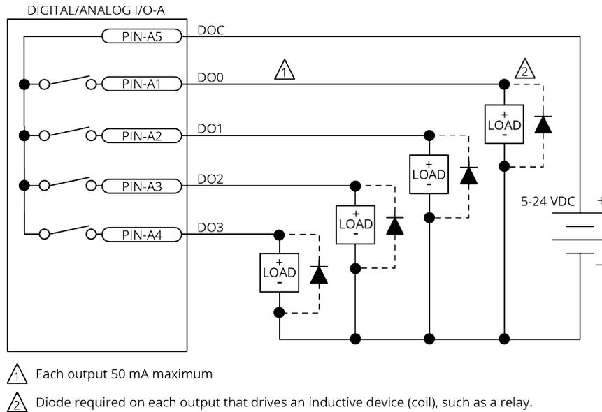
**Figure 2-17: Digital Outputs Connected in Current Sourcing Mode**
