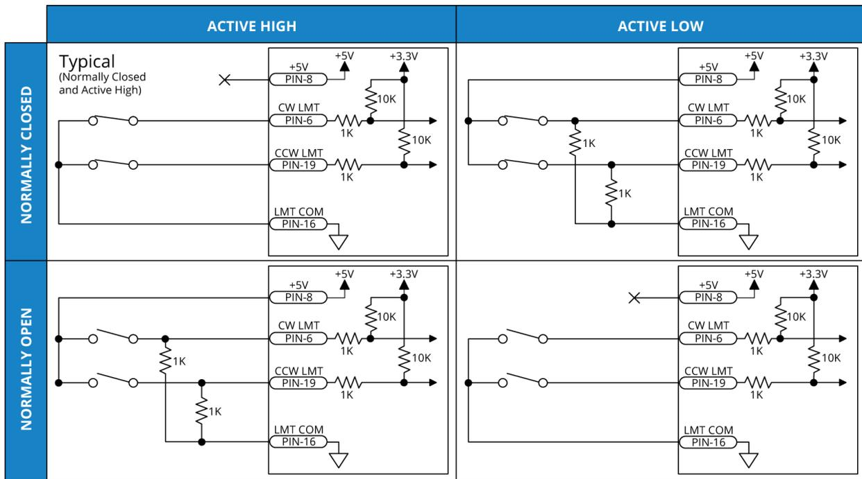
Figure 2-13: End of Travel Limit Input Connections
