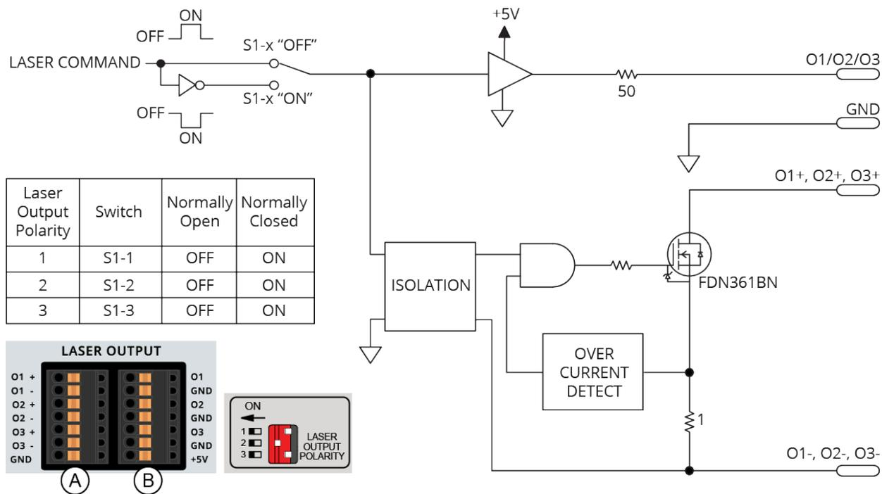
**Figure 2-5: Laser Interface Outputs**
