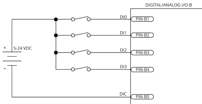
**Figure 2-19: Digital Inputs Connected to Current Sourcing Devices**
