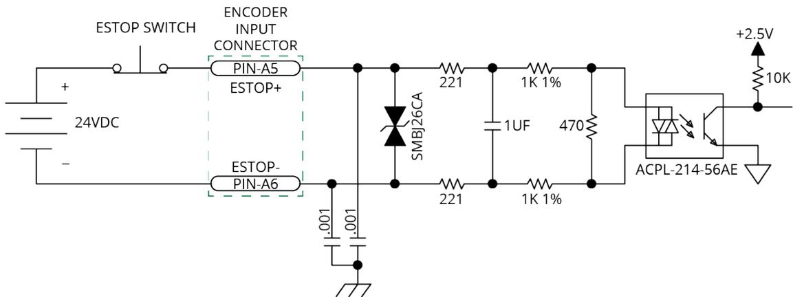
Figure 2-24: ESTOP Sense Input Schematic
