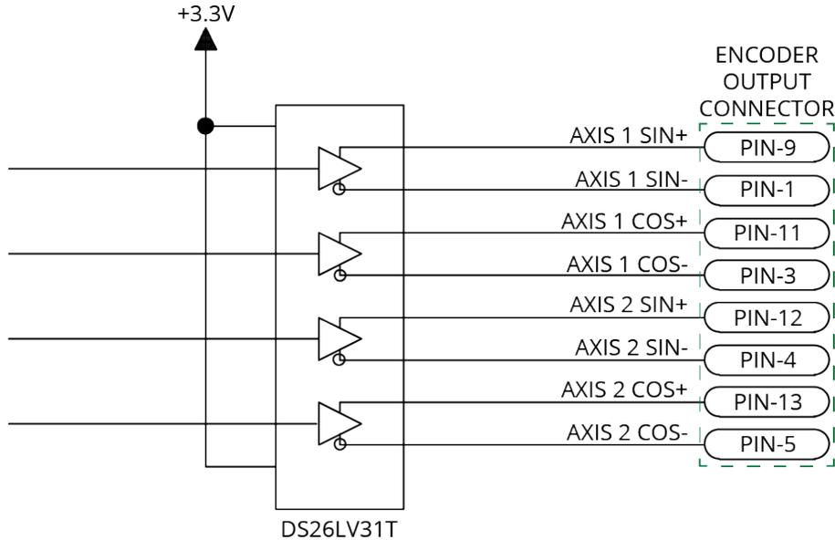
**Figure 2-11: Encoder Outputs**
