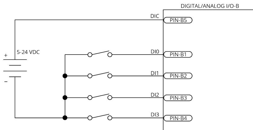
**Figure 2-20: Digital Inputs Connected to Current Sinking Devices**
