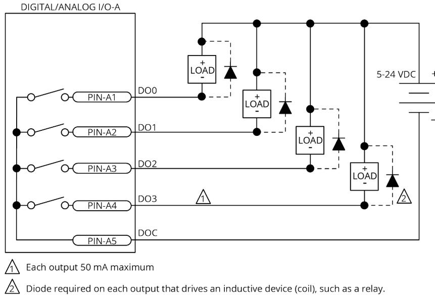
**Figure 2-18: Digital Outputs Connected in Current Sinking Mode**
