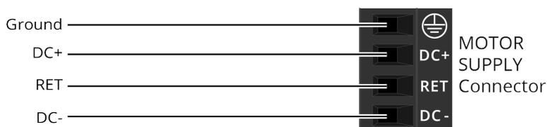
**Figure 2-2: Motor Supply Connections**
