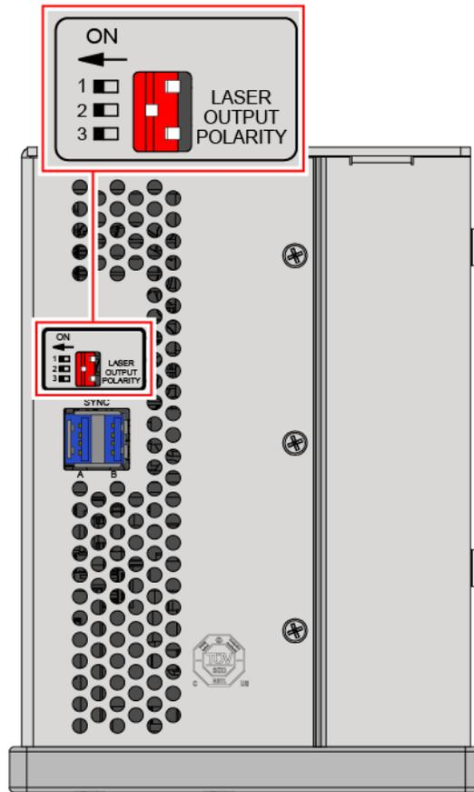
Figure 2-25: Laser Output Polarity Switches
