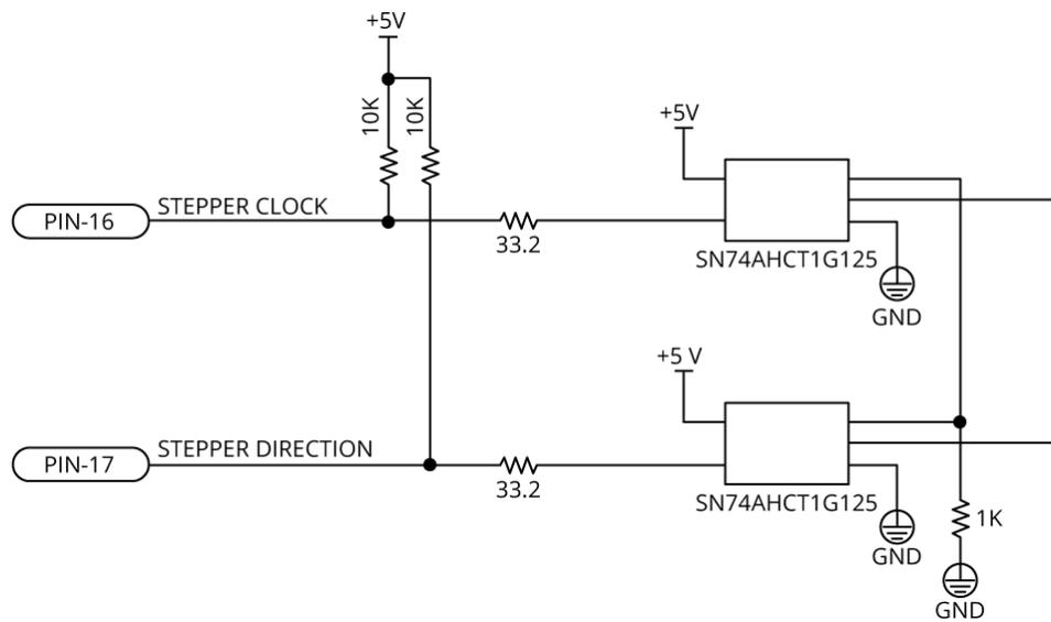
**Figure 2-3: Stepper Clock and Stepper Direction Output Schematic**
