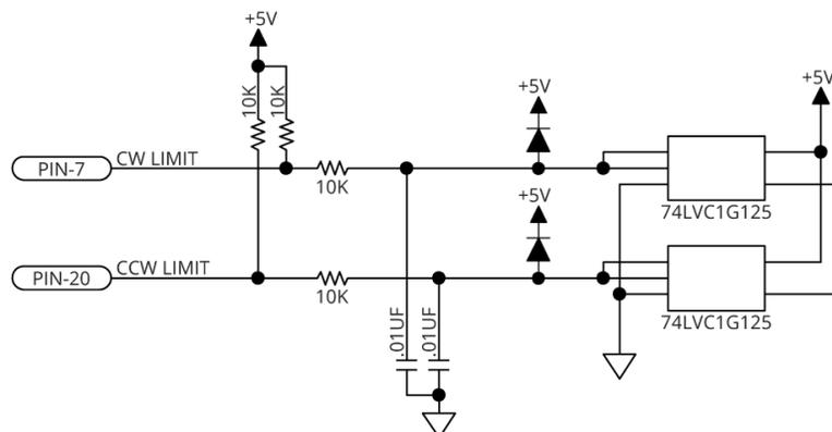
**Figure 2-5: End of Travel Limit Input Schematic**
