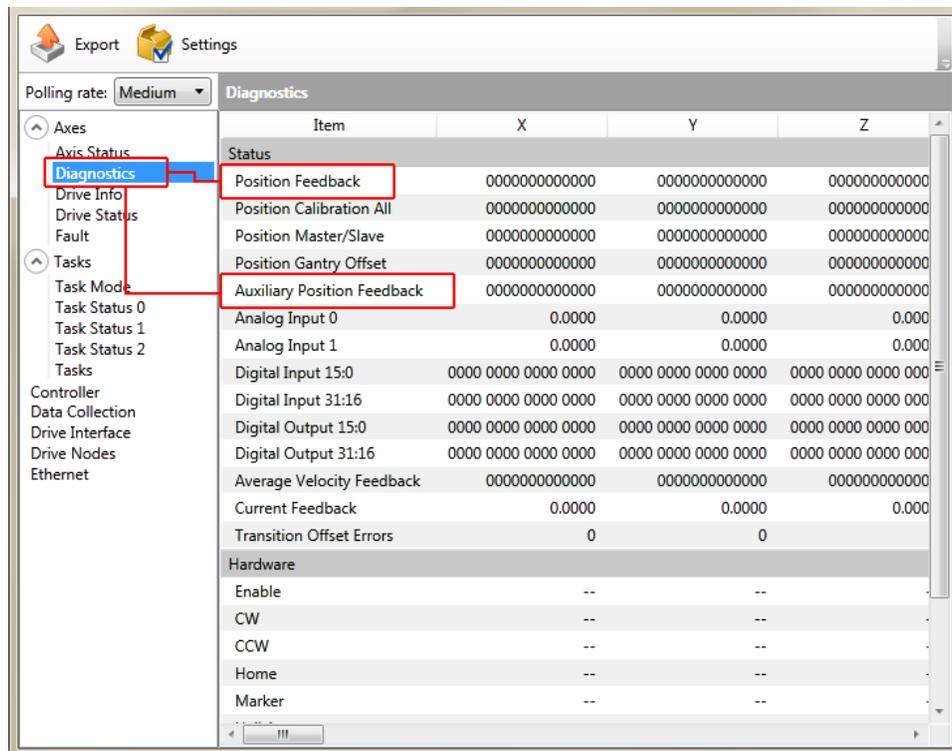
**Figure 2-12: Position Feedback in the Diagnostic Display**
