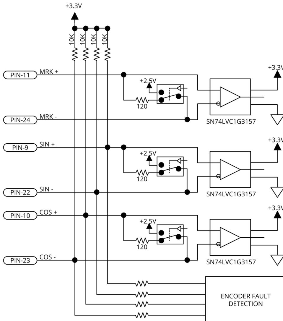
**Figure 2-9: Square Wave Encoder Schematic (Axis Connector)**
