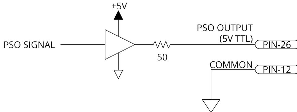
**Figure 2-21: PSO TTL Outputs Schematic**
