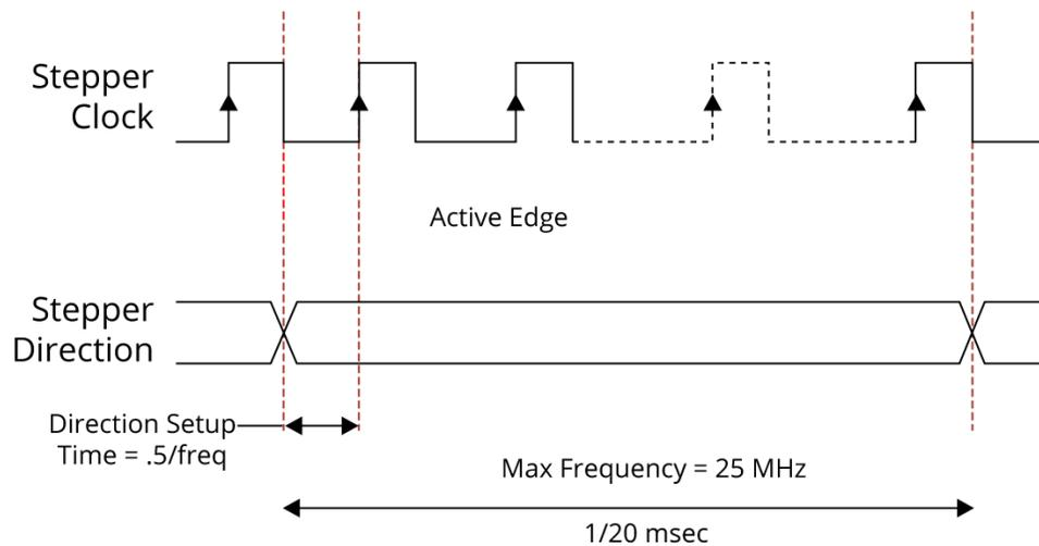
**Figure 2-2: Stepper Clock and Stepper Direction Timing**
