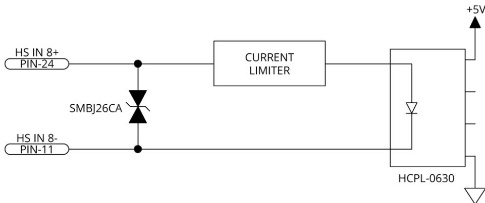
**Figure 2-20: High-Speed Input**
