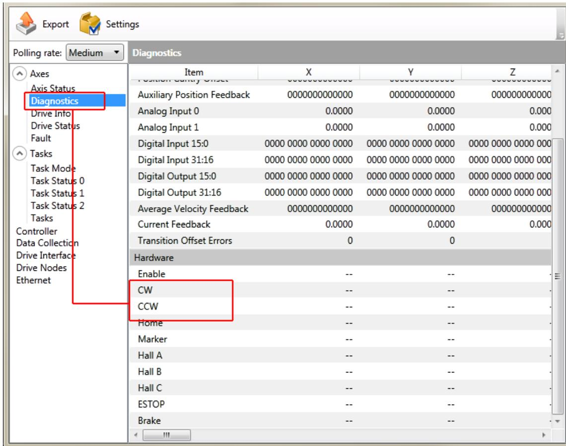
**Figure 2-6: End of Travel Limit Input Diagnostic Display**
