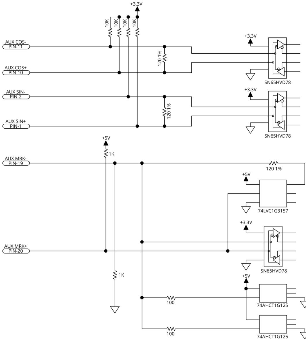
**Figure 2-28: Square Wave Encoder Interface (Aux I/O Connector)**
