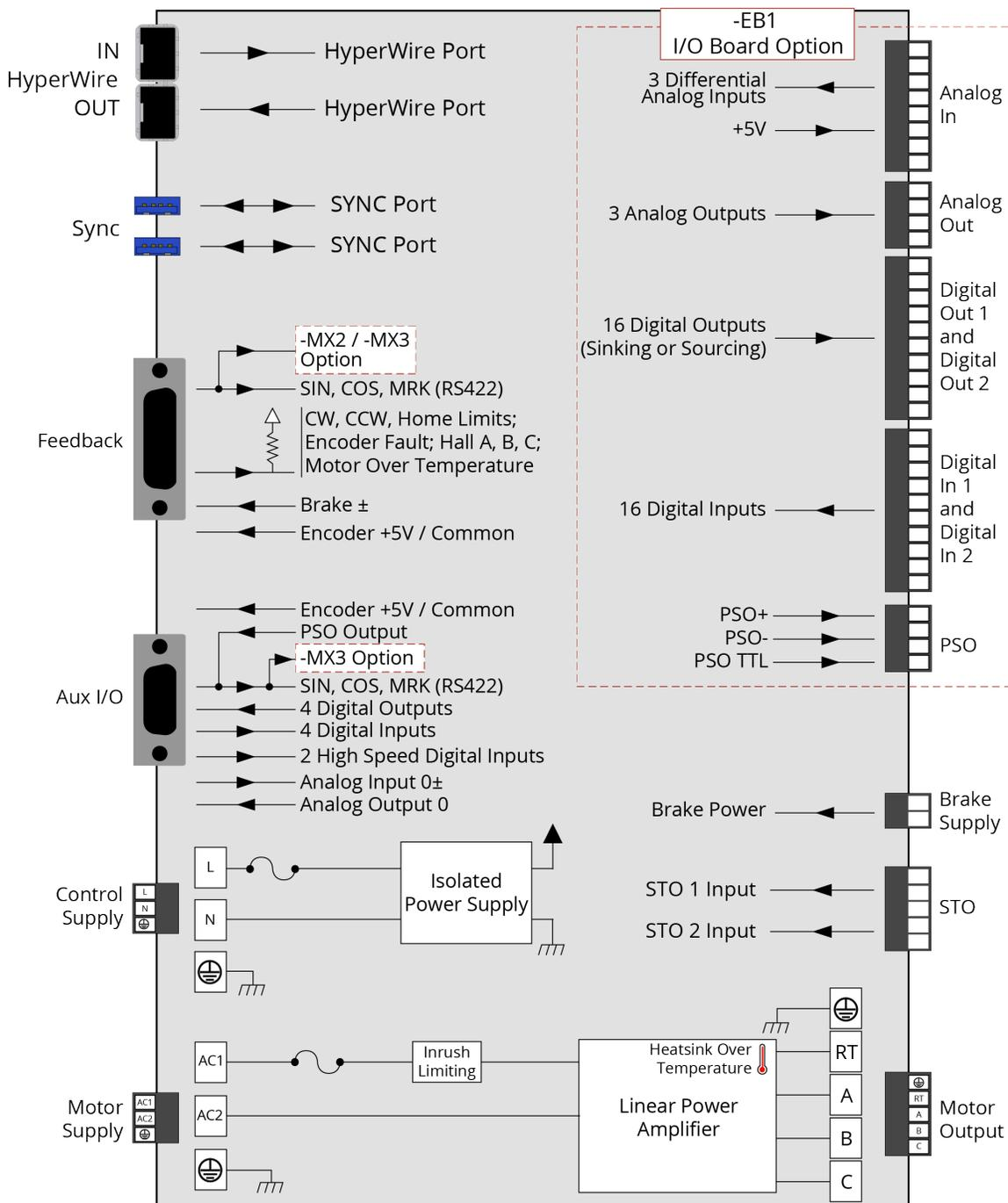
Figure 1-2: Functional Diagram
