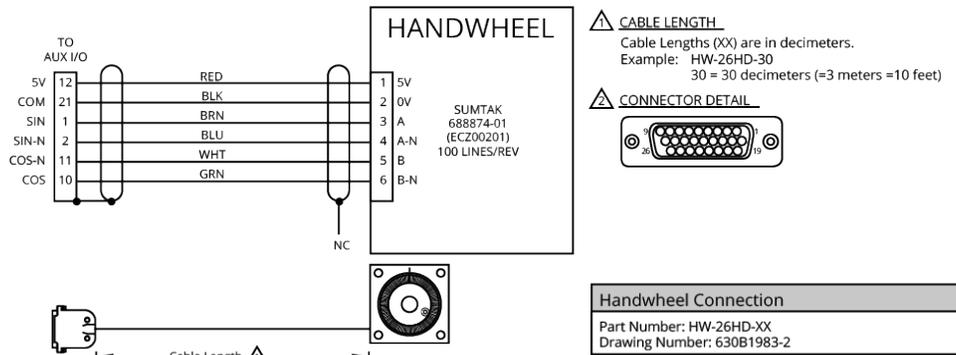
**Figure 4-3: Handwheel Interconnection to Aux I/O Connector**
