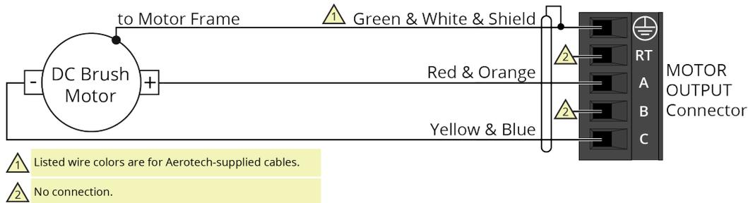
Figure 2-8: DC Brush Motor Configuration
