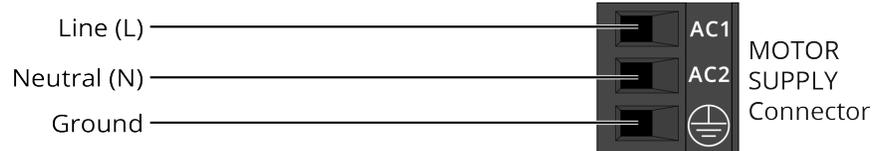
Figure 2-2: Motor Supply Connections
