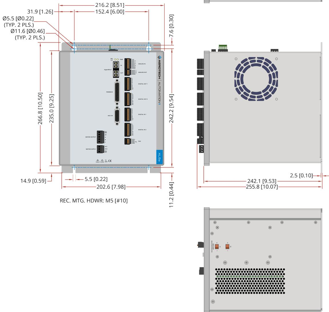
Figure 1-4: Dimensions [-EB1]
