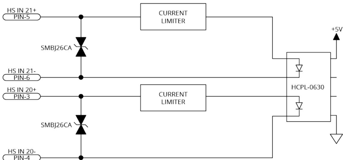
**Figure 2-39: High-Speed Inputs**
