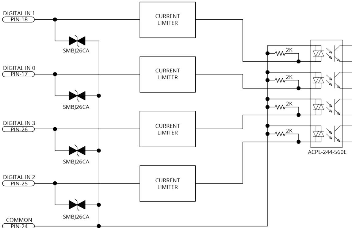
**Figure 2-36: Digital Inputs Schematic (Aux I/O Connector)**
