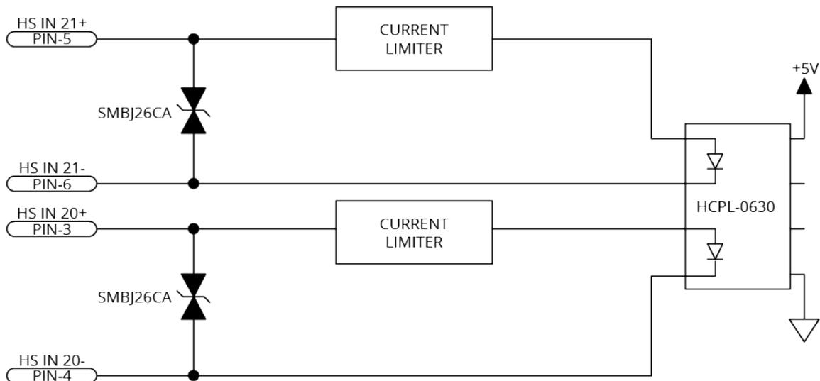
**Figure 2-42: High-Speed Inputs**
