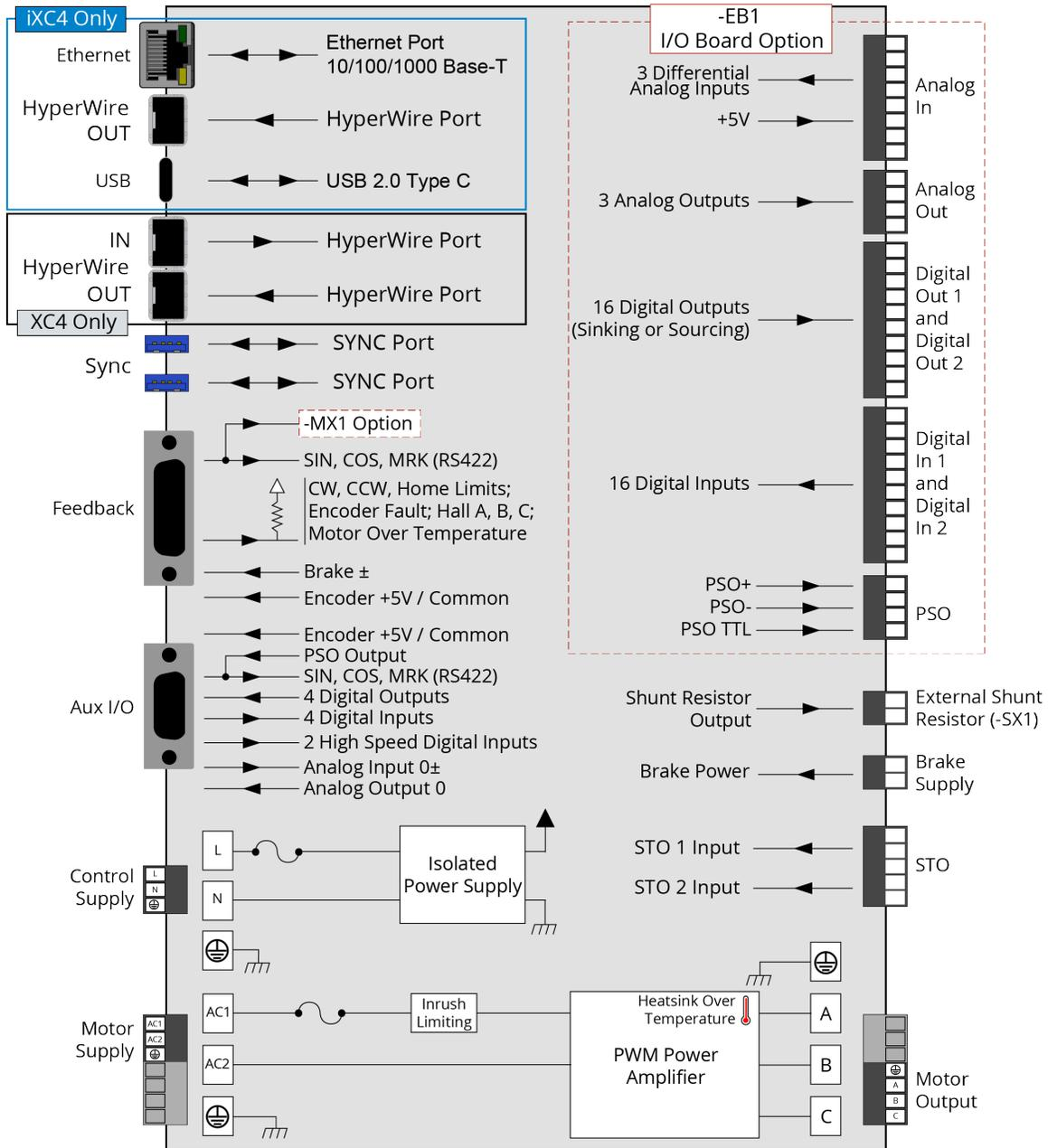
Figure 1-3: Functional Diagram
