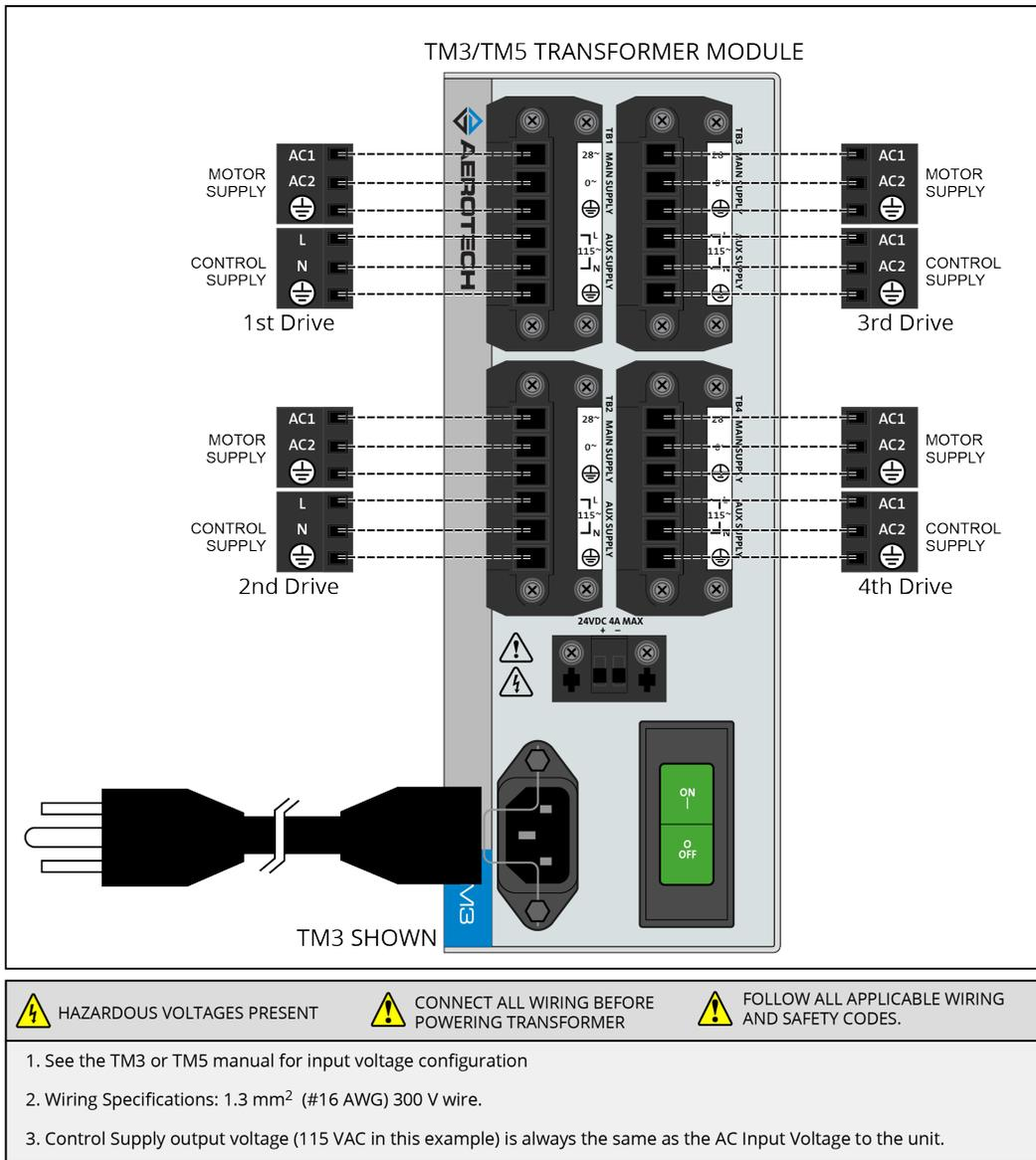
**Figure 2-8: TM3/TM5 Transformer Control and Motor Power Wiring**
