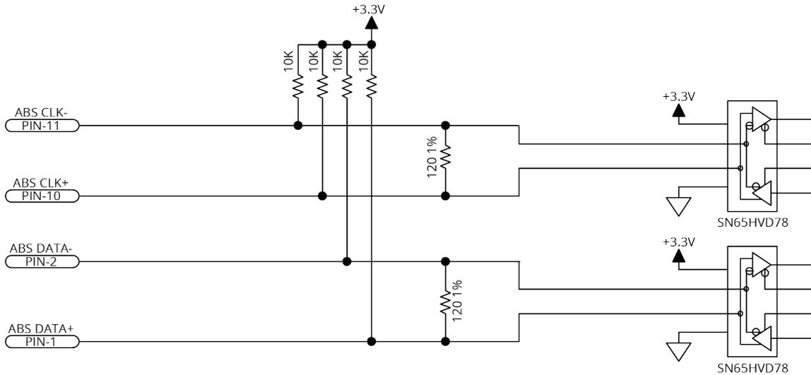
**Figure 2-34: Absolute Encoder Schematic (Auxiliary I/O Connector)**
