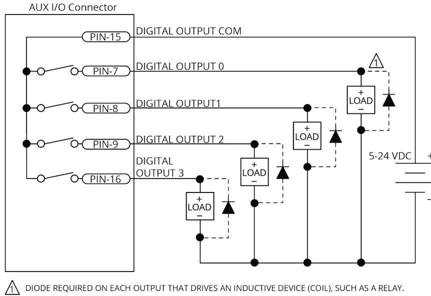
**Figure 2-37: Digital Outputs Connected in Current Sourcing Mode**
