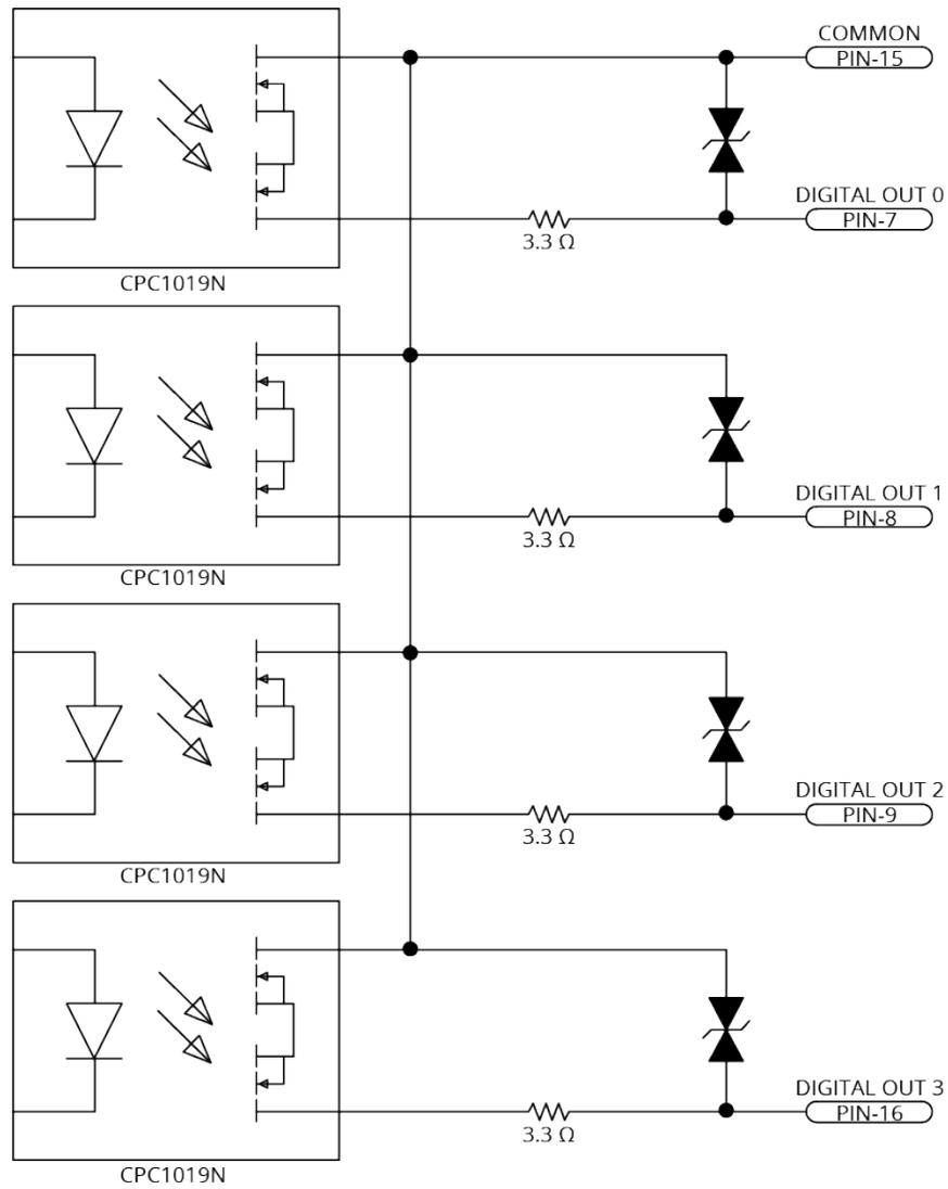
**Figure 2-36: Digital Output Schematic (Aux I/O Connector)**
