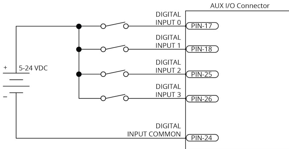
**Figure 2-40: Digital Inputs Connected to Current Sourcing Devices**
