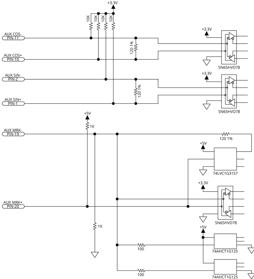
**Figure 2-33: Square Wave Encoder Interface (Aux I/O Connector)**
