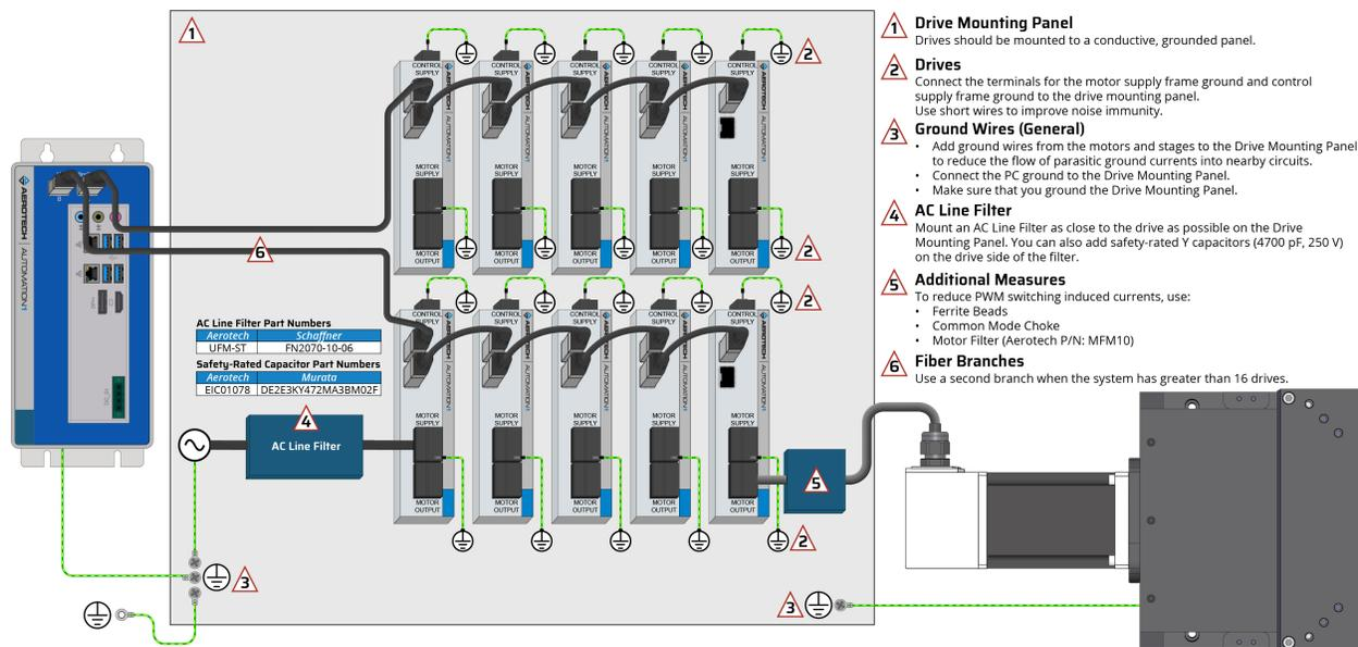
Figure 2-46: PC-Based System Wiring Drawing (Best Practice)
