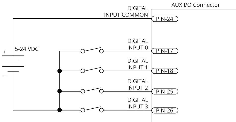
**Figure 2-41: Digital Inputs Connected to Current Sinking Devices**
