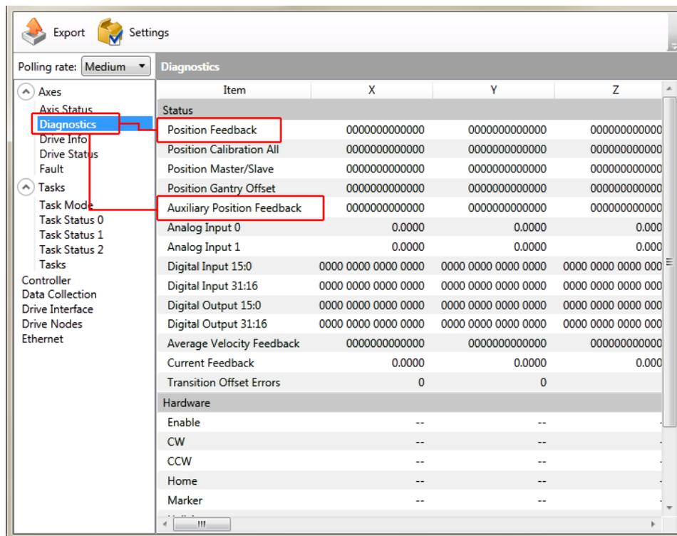
**Figure 2-23: Position Feedback in the Diagnostic Display**
