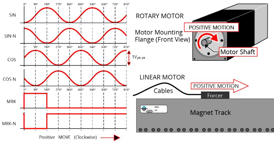
**Figure 2-20: Sine Wave Encoder Phasing Reference Diagram**
