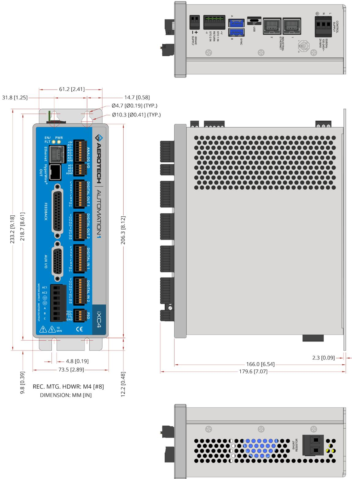
Figure 1-5: Dimensions [-EB1]
