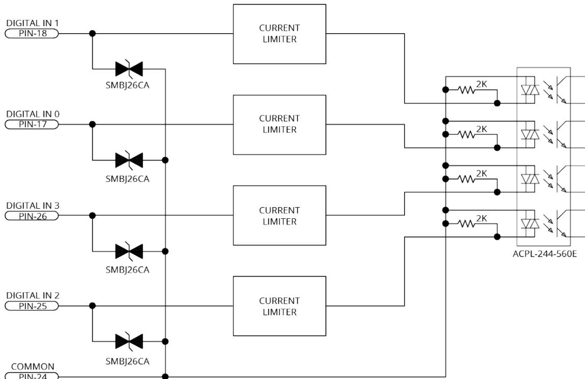
**Figure 2-39: Digital Inputs Schematic (Aux I/O Connector)**
