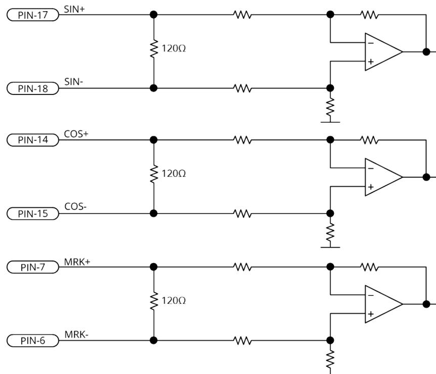
**Figure 2-21: Sine Wave Encoder Schematic (Feedback Connector)**
