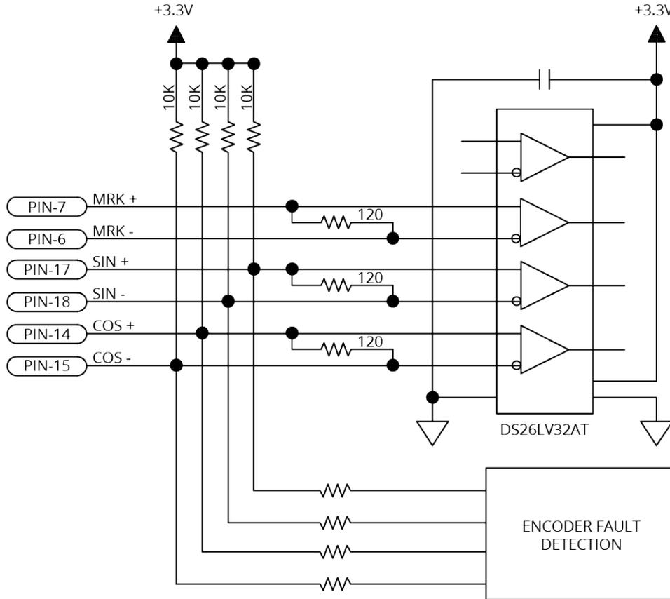
**Figure 2-18: Square Wave Encoder Schematic (Feedback Connector)**
