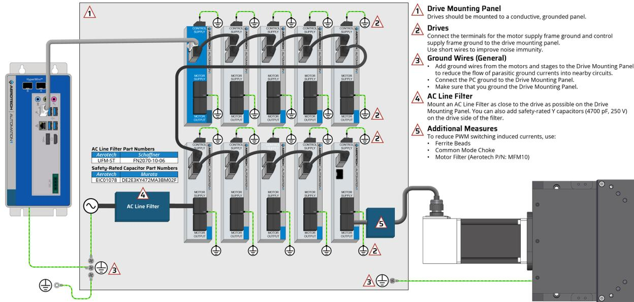
Figure 2-45: Drive-Based System Wiring Drawing (Best Practice)
