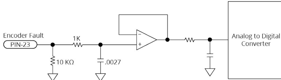
**Figure 2-26: Encoder Fault Input Schematic (Feedback Connector)**
