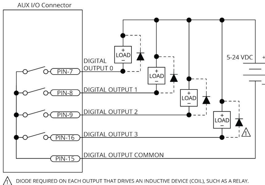
**Figure 2-38: Digital Outputs Connected in Current Sinking Mode**
