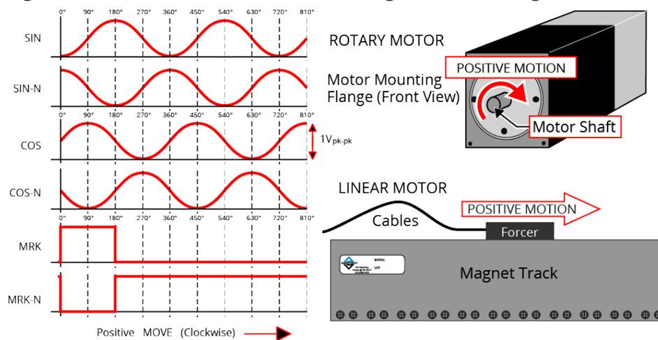
**Figure 2-15: Sine Wave Encoder Schematic (Feedback Connector)**
