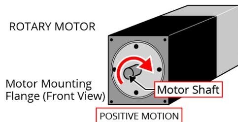
4. If the voltmeter indicates a negative value, swap the motor leads and move the motor by hand in the positive direction, again. When the voltmeter indicates a positive value, the motor leads have been identified.
