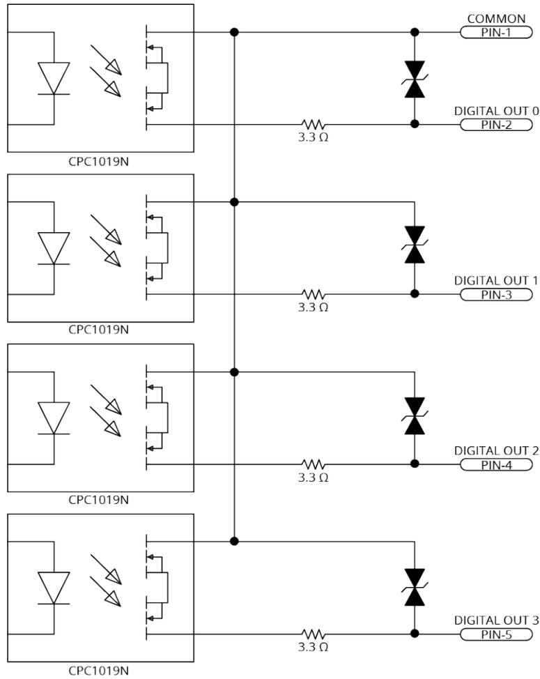
**Figure 3-9: Digital Outputs Connected in Current Sourcing Mode [-EB1]**
