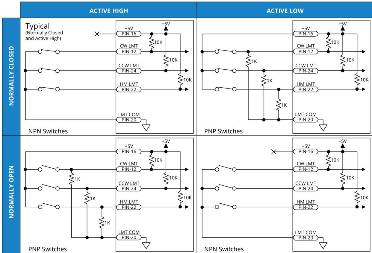
Figure 2-22: End of Travel and Home Limit Input Schematic (Feedback Connector)
