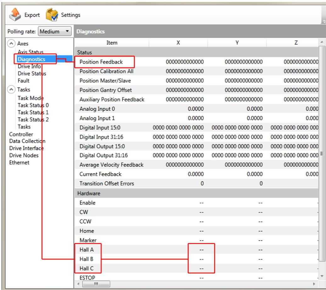
**2.2.1.2. Brushless Motor Unpowered Motor and Feedback Phasing**
