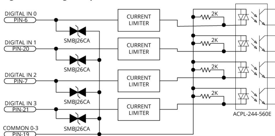
Each group of four inputs must be connected in an all sourcing or all sinking configuration.
