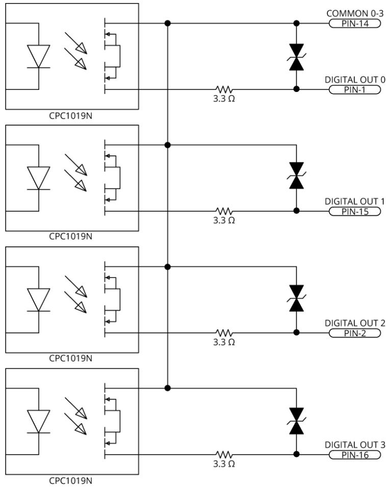
**Figure 2-4: Digital Outputs Connected in Current Sourcing Mode**
