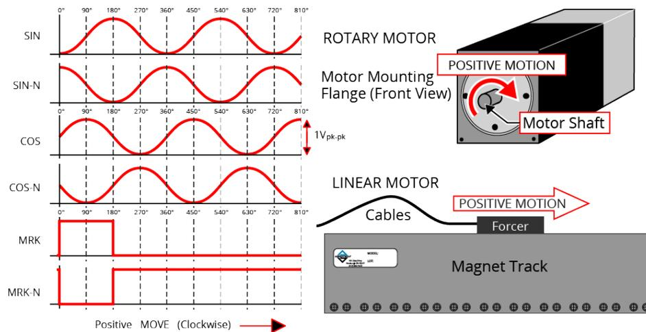
**Figure 2-23: Sine Wave Encoder Schematic (Feedback Connector)**
