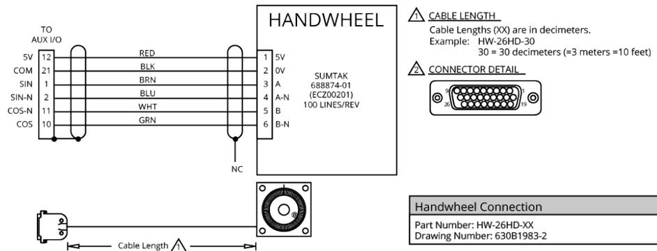
**Figure 4-4: Handwheel Interconnection to the Aux I/O through a BBA32 Module**
