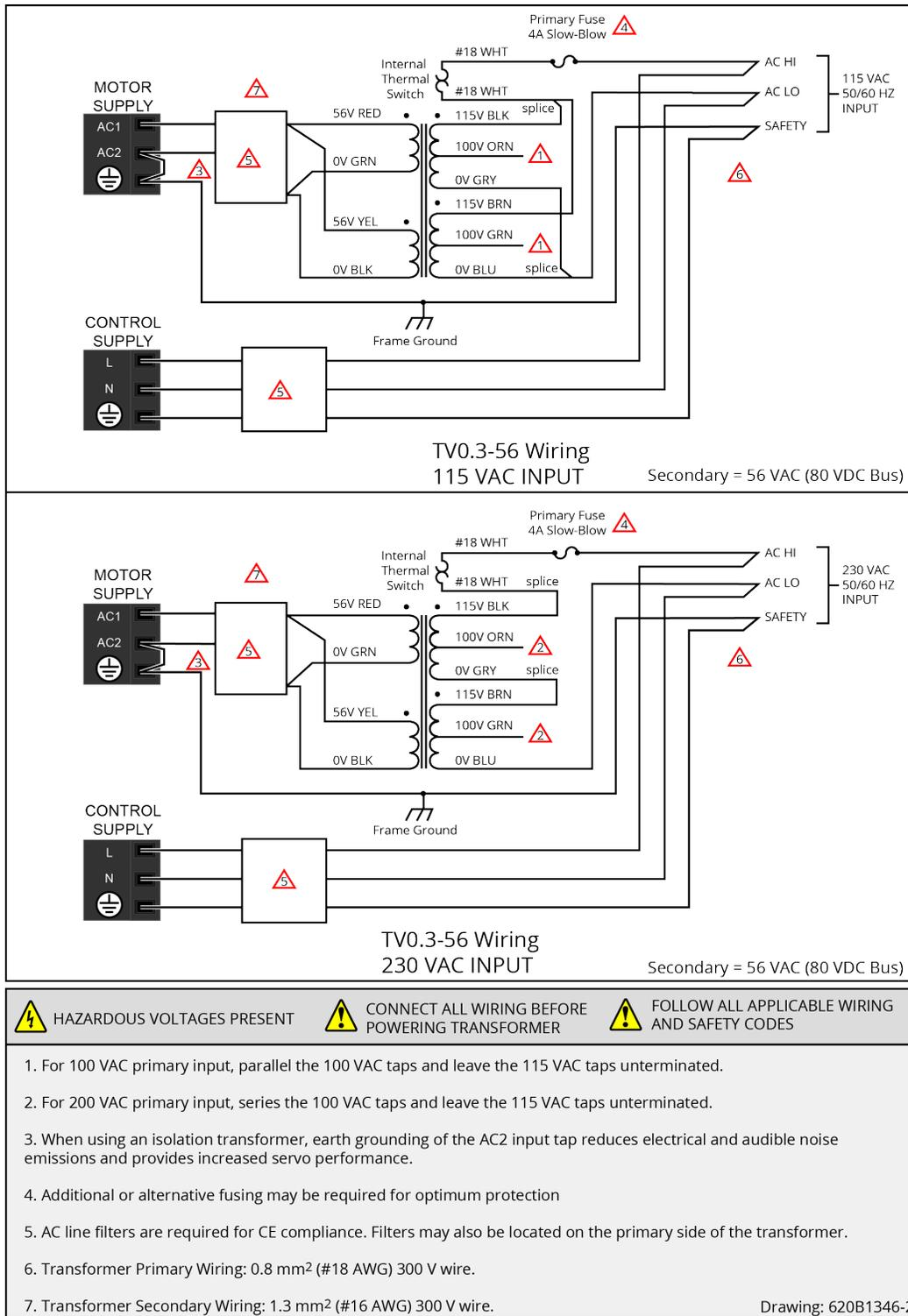
Figure 2-8: TM3/TM5 Transformer Control and Motor Power Wiring
