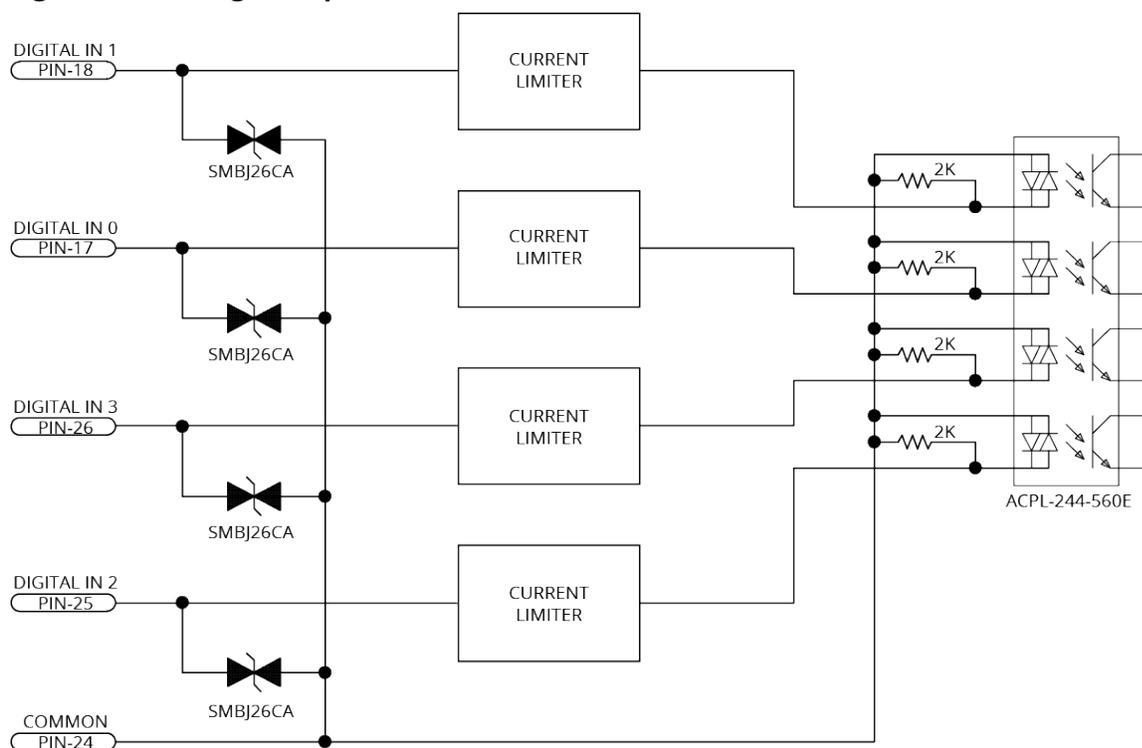
**Figure 2-44: Digital Inputs Connected to Current Sourcing Devices**
