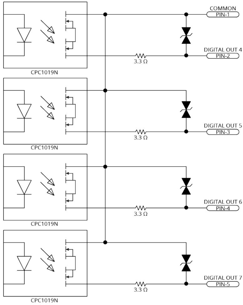
**Figure 3-3: Digital Outputs Connected in Current Sourcing Mode [-EB1]**
