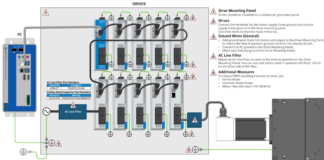
Figure 2-50: PC-Based System Wiring Drawing (Best Practice)
