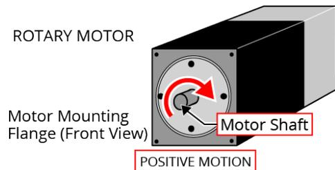
4. If the voltmeter indicates a negative value, swap the motor leads and move the motor by hand in the positive direction, again. When the voltmeter indicates a positive value, the motor leads have been identified.
