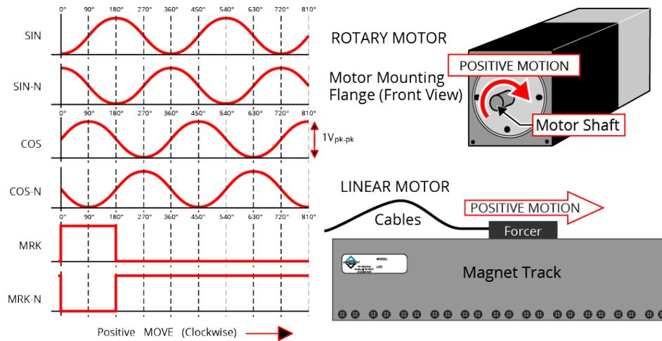
**Figure 2-38: Sine Wave Encoder Schematic (Auxiliary I/O Connector)**
