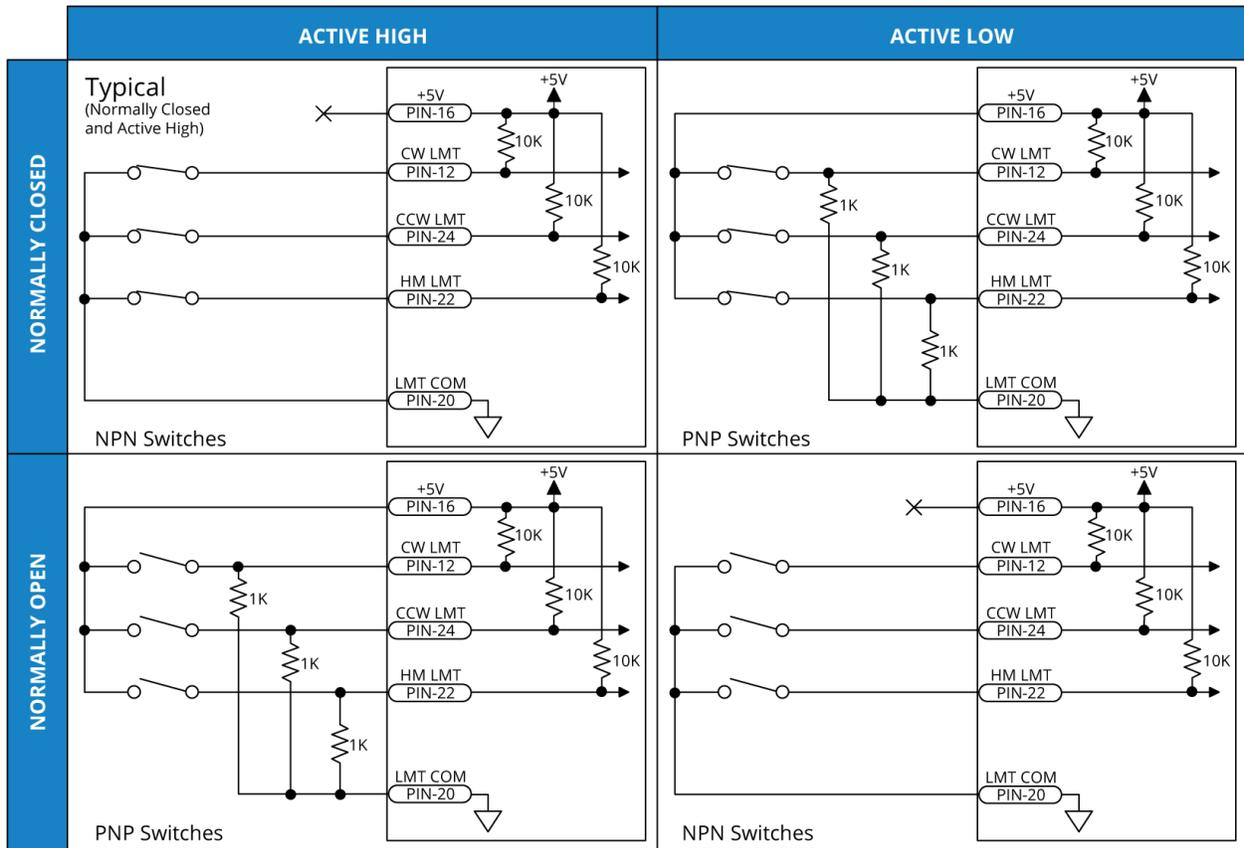
Figure 2-30: End of Travel and Home Limit Input Schematic (Feedback Connector)
