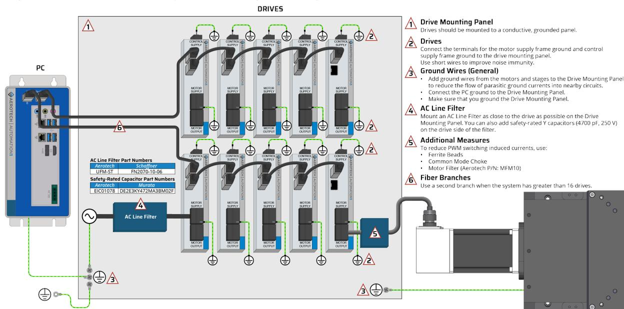
Figure 2-51: Drive-Based Controller System Interconnection (Best Practice)
