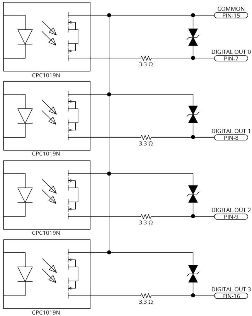
**Figure 2-41: Digital Outputs Connected in Current Sourcing Mode**
