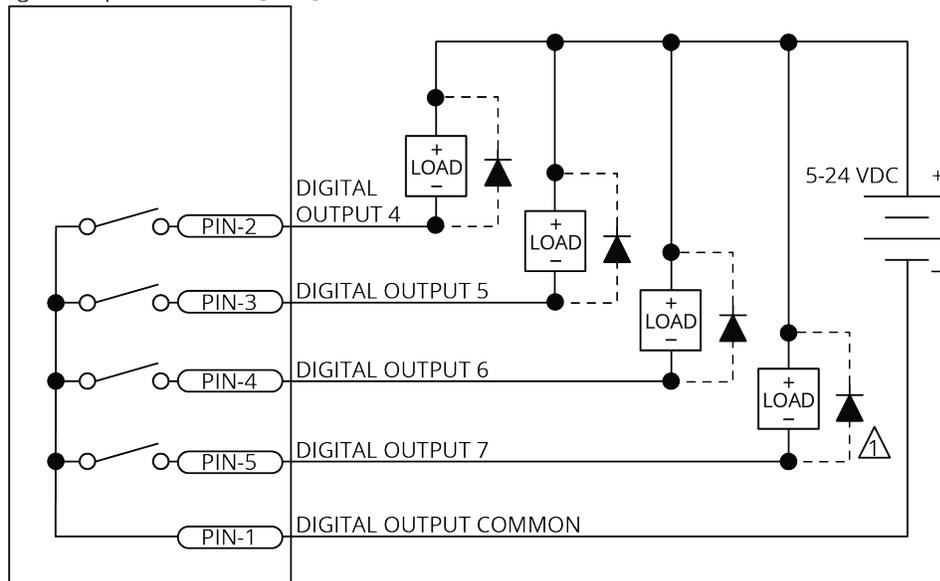
DIODE REQUIRED ON EACH OUTPUT THAT DRIVES AN INDUCTIVE DEVICE (COIL), SUCH AS A RELAY.
