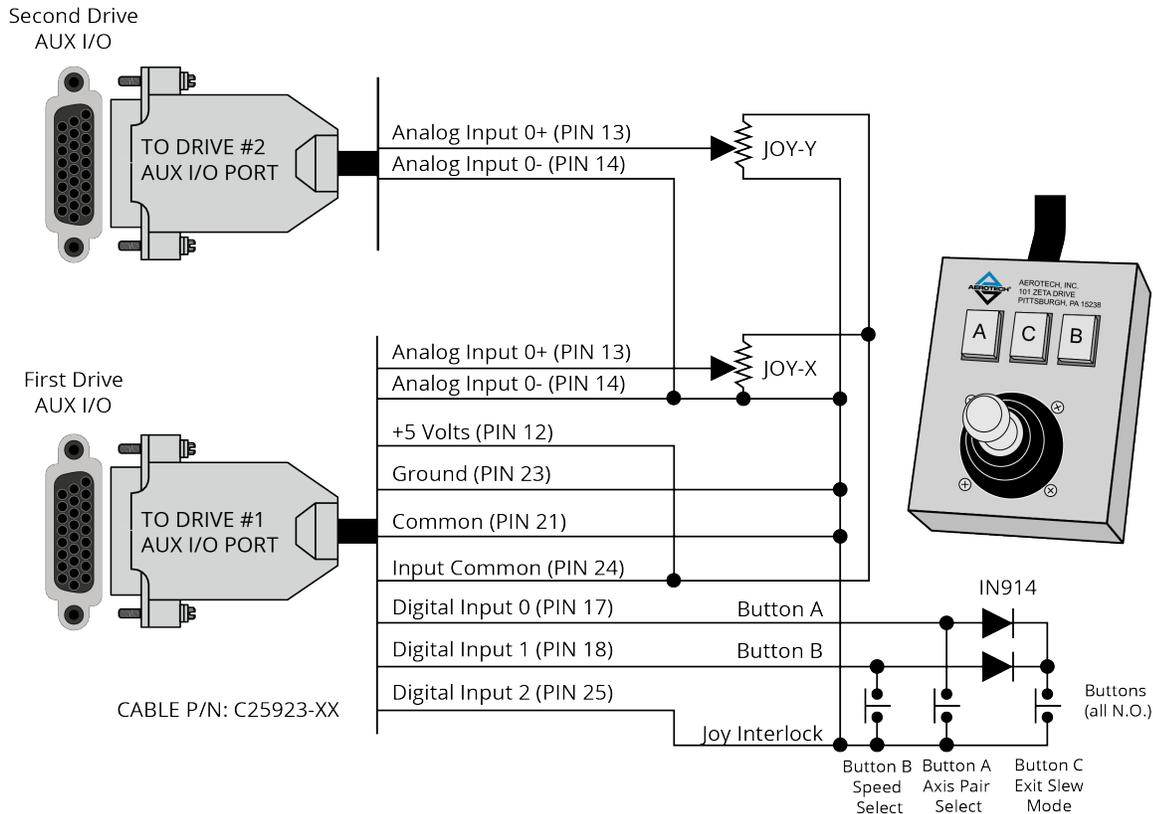
Figure 4-2: Two Axis Joystick Interface (to the I/O board)
