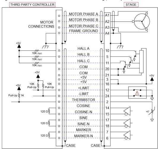
Figure 3-2: ANT130XY Motor and Feedback Wiring [-CN2 Option]
